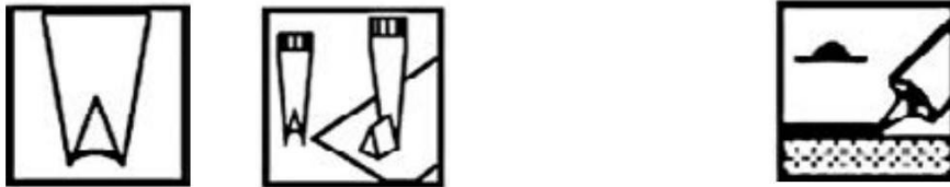
Obr. 36 Tvar housenky lepidla Sikaflex 552 / SikaFast 555 L10 [28]
