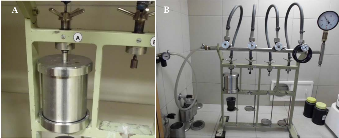
Fig. 25: Chamber with the filtration barrier (A) and panorama of the filtration station (B)
