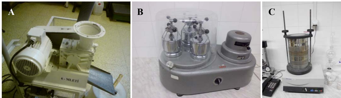
Fig. 16: Laboratory jaw crusher (A), planetary ball mill (B) and sieving vibration analyzer AS 200 digit (C)
