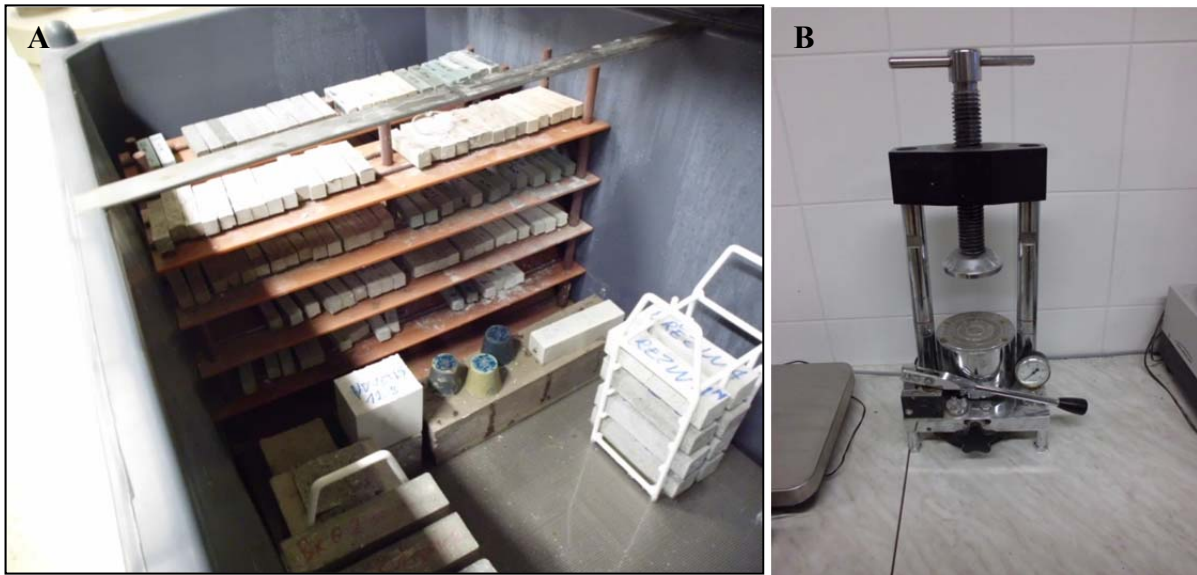
Fig. 19: Water bath for storage of samples (A) and laboratory press (B)
