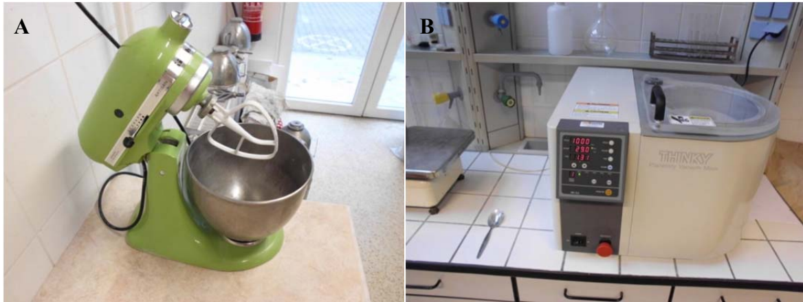
Fig. 18: Laboratory mechanical mixer (A) and vacuum mixer Thinky (B)
