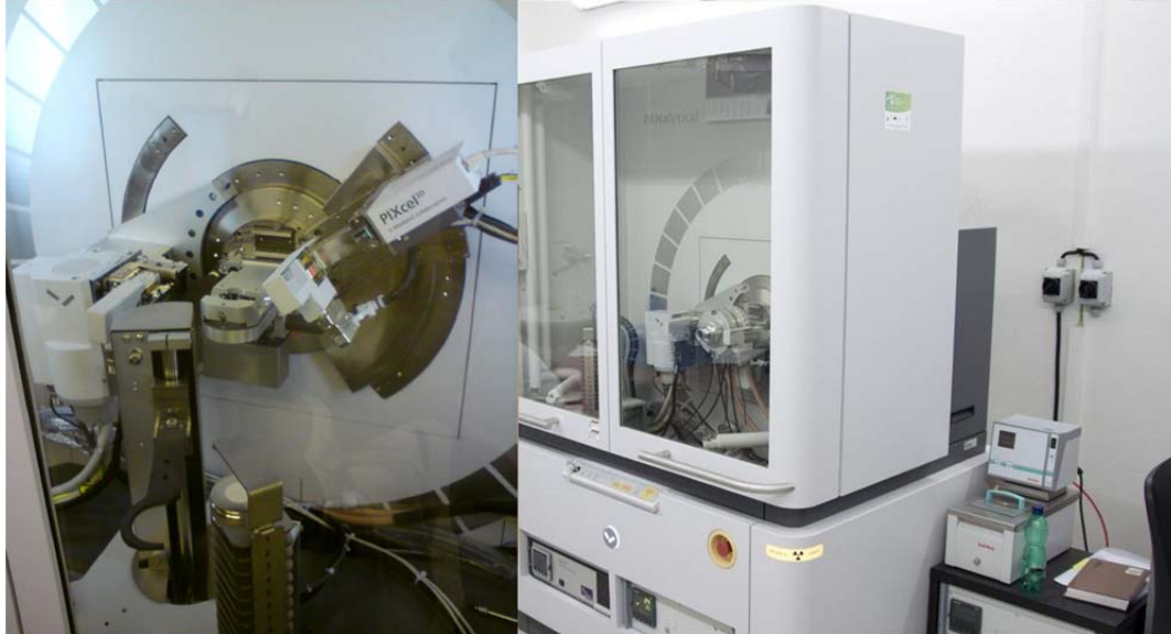
Fig. 23: XRD spectrometer PANalytical Empyrean
