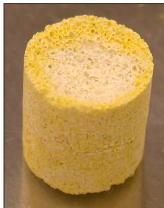
Fig. 2.5: The continuous BeO structure after removing the uranium [41].
