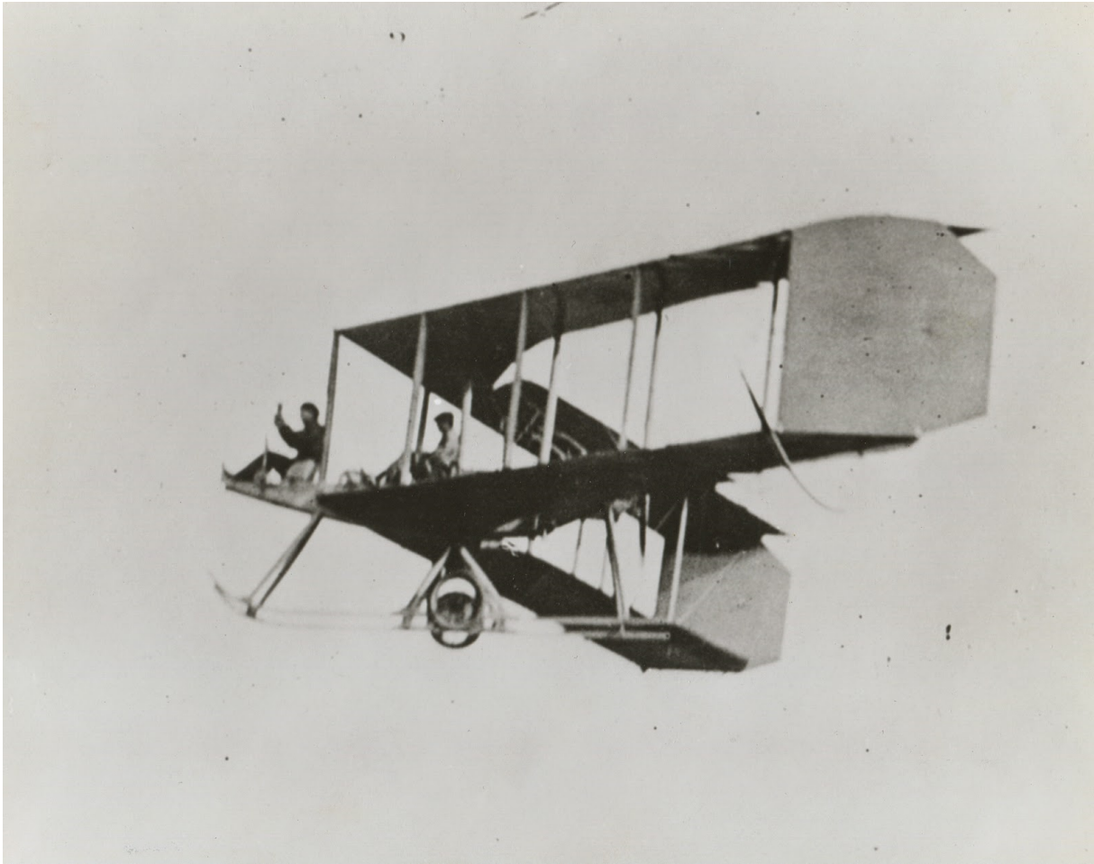
Figure 4.2: Bruggess Dunne BD-1B - designed by John William Dunne [28]
