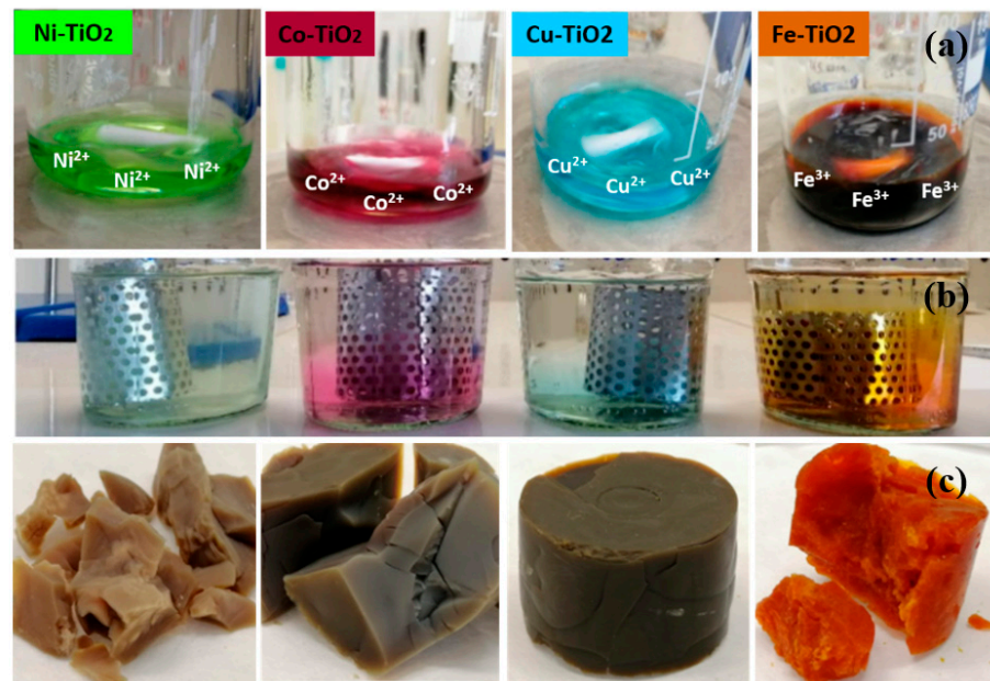
Figure 1. (a) The process of synthesis of the metal-doped \text{TiO}_2 aerogels prepared with the metal acetate precursor of \text{Ni}^{2+} , \text{Co}^{2+} , \text{Cu}^{2+} , \text{Fe}^{3+} ions. (b) Involving the gelation of the alcogels followed by solvent exchange with acetone. (c) Finally, supercritical drying to obtain aerogel samples.
