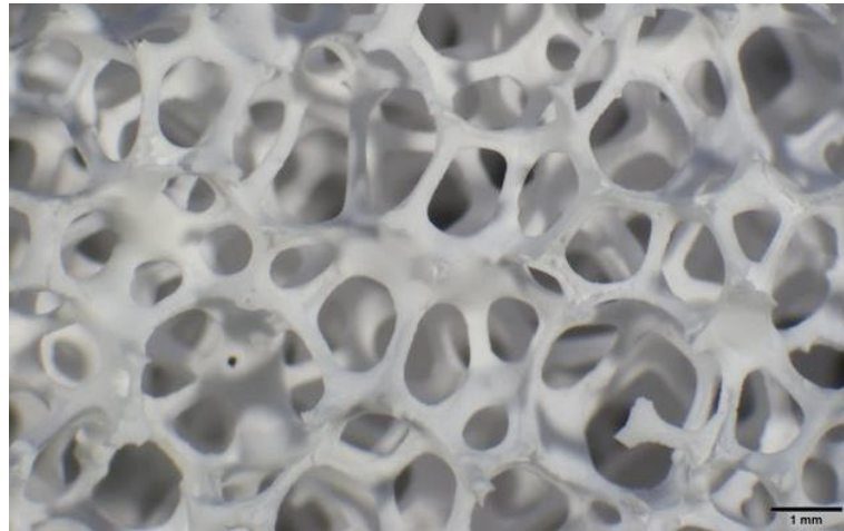
Fig. 3 Macrostructure of alumina foam (A7250)
