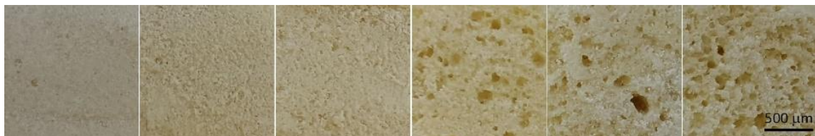
Fig. 22 CaP/PU foams having \text{ha/pu ratio} = 1 and I_{\text{NCO}} = 105 (water content increasing from 0 wt.% (left) to 5 wt.% (right) of polyol)
