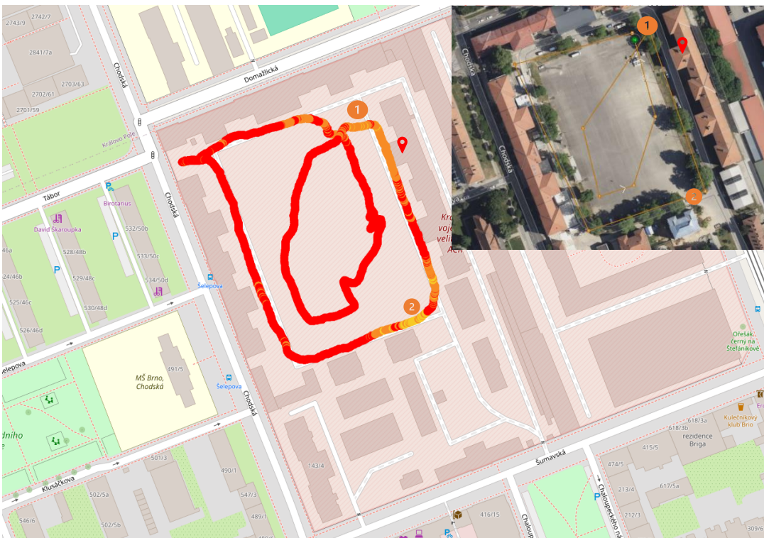
Fig.6.10 The coverage of the BS at Šumavská barrak in the real flight test, altitude 15 m, the figure at the top-right is the preset waypoints in QGroundControl.
