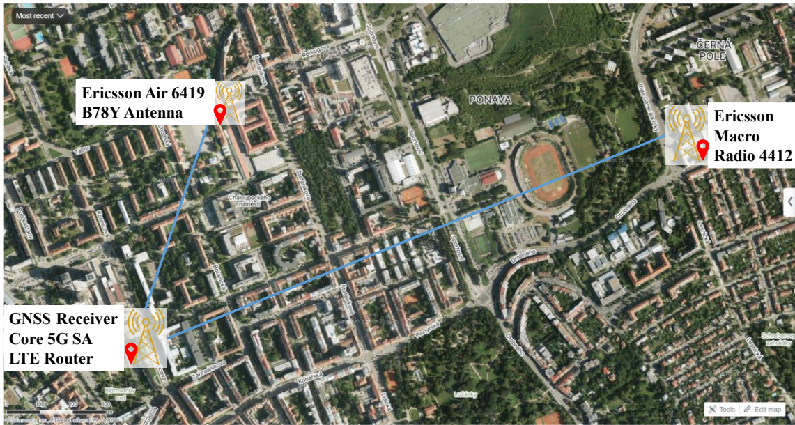
Fig.2.7 Private 5G SA network setup at UNOB, blue lines are illustrated for optical links, edited from mapy.cz
