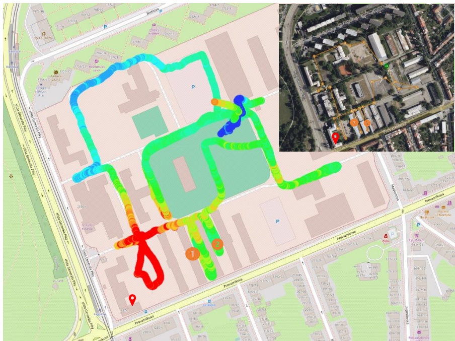
Fig.6.8 The coverage of the BS at Černá Pole barracks in the real flight test, altitude 15 m, the figure at the top-right is the preset waypoints in QGroundControl
