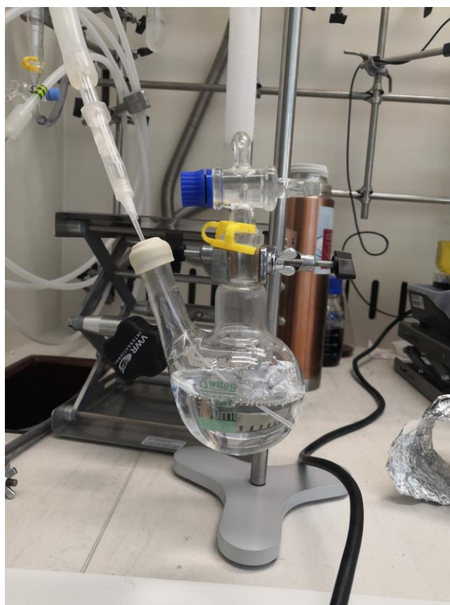
Figure 16. Apparatus for water stripping.
