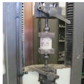
Figure 3. Heckert FPZ 100/1 mechanical press for the direct tensile strength test (specimen 8C_P3).
