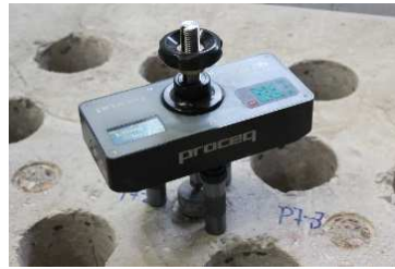
Figure 1. Proceq DY-216: pull-off bond strength automated tester.
