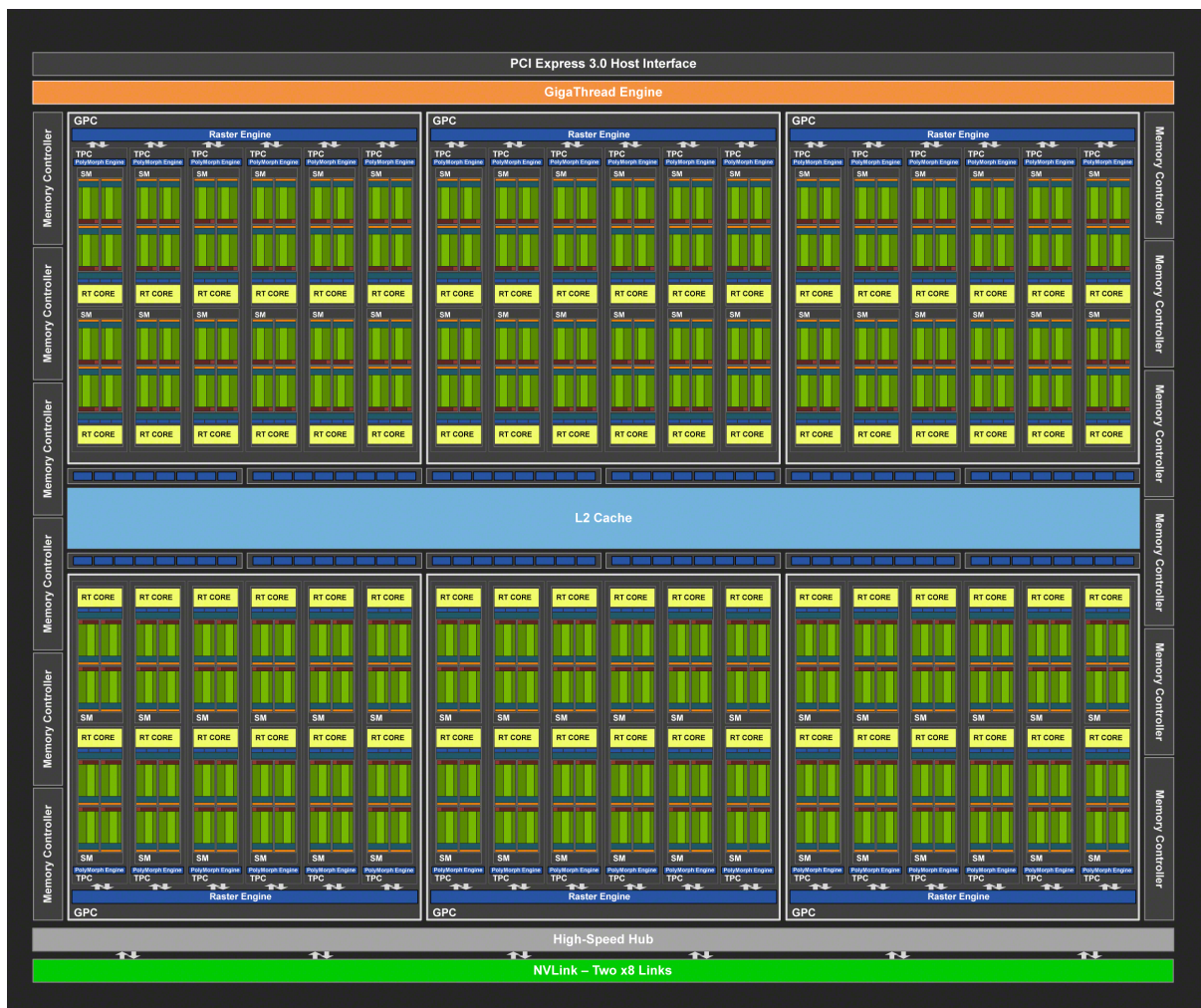
Obr. 4: GPU architektura NVIDIA Turing – čip TU102 [62].
