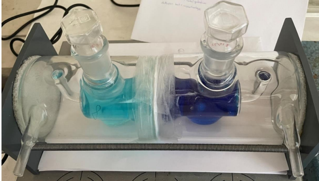
Figure 33. Measurement of the diffusion coefficient on side-bi-side cells with a membrane consisting of 8 layers of non-woven fabric connected by 3% (w/w) gelatine hydrogel after 8 hours.
