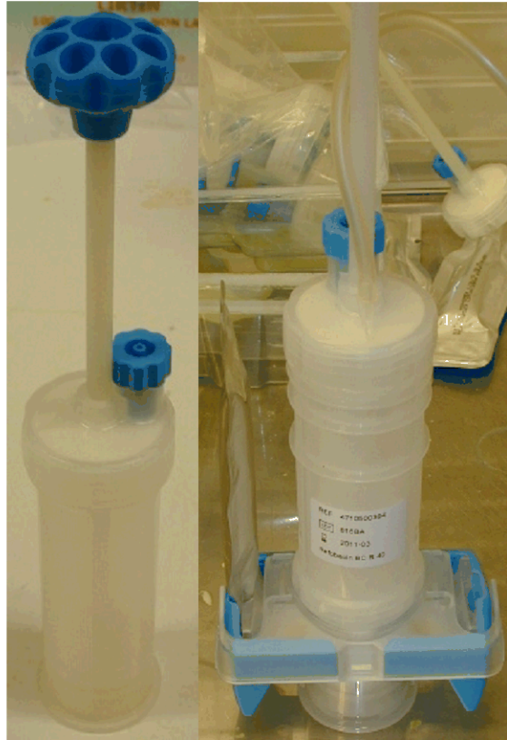
Figure 2.3.4.: Optivac (left) and Optipac (right) mixing system.
