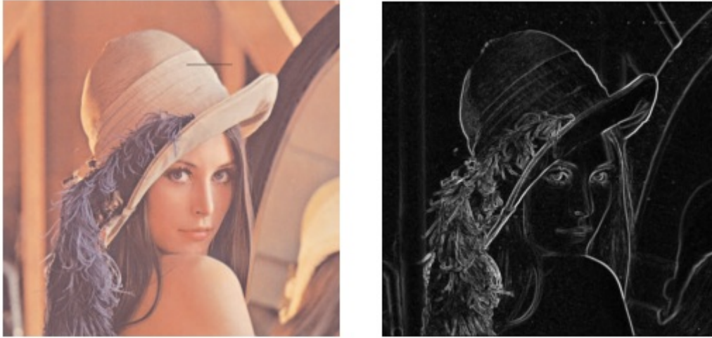
Fig. 5. Example of colour morphological gradient operator for edge detection [5]
