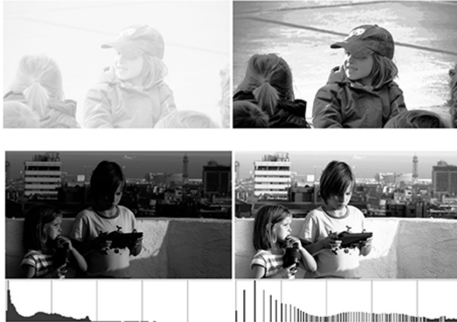
Fig. 4. Application of histogram equalization on the left images. Top one represents a bad equalization as the image was overexposed The bottom is then a good example of equalization [4]
