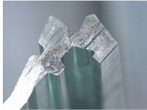
Figure 2.5: Fatigue cracks on core 532
