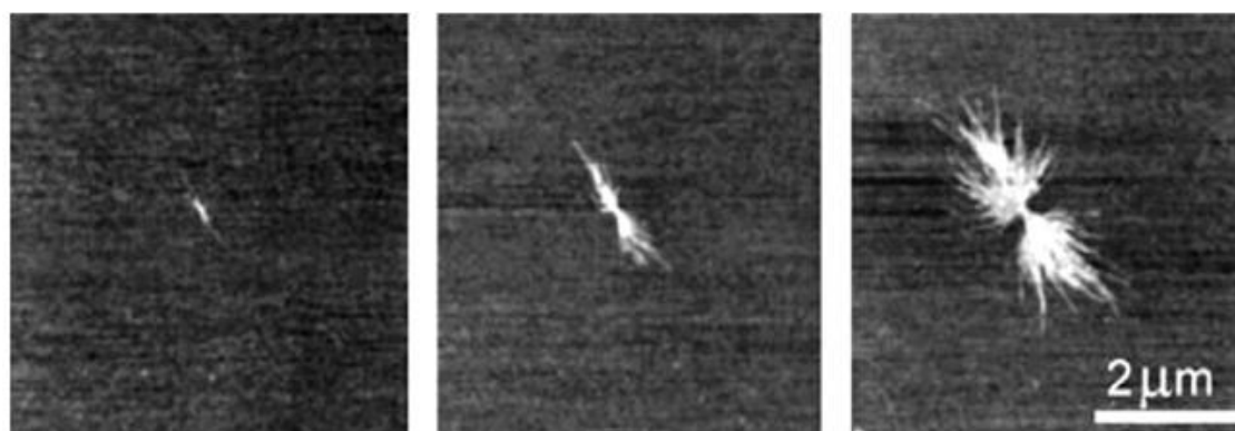
Figure 5: In situ AFM recording of a homogeneous nucleation [42].
