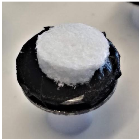
Figure 8 – A scaffold sample attached to an aluminium pin stub with the carbon tape.
