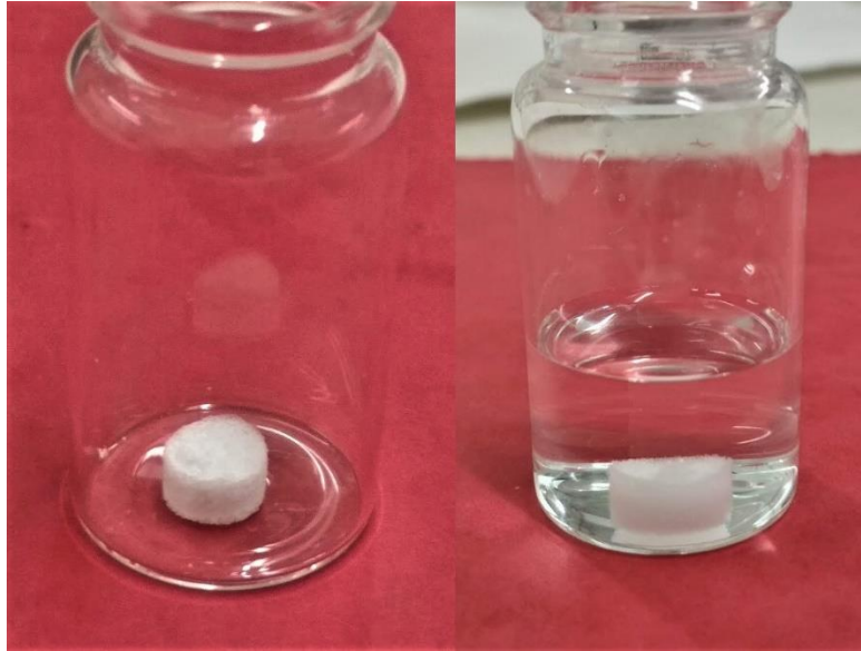
Figure 9 – A scaffold sample before (left) and after (right) immersion in PBS solution in the swelling behaviour and enzymatic degradation analyses.
