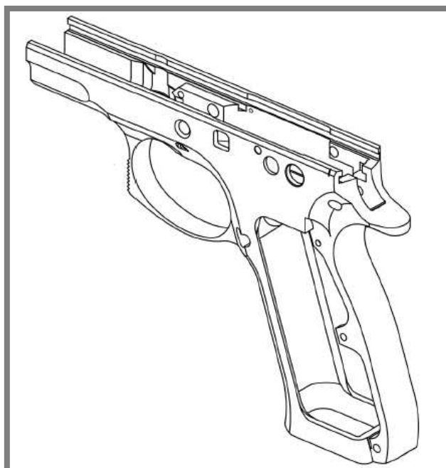
Obr. 1-4 Rám pistole CZ 75D Compact [2]
