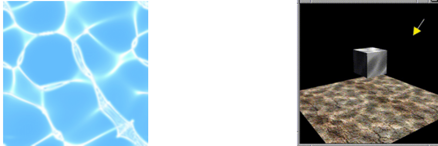
Figure 5.2: Caustics patterns created using Stam’s approach [89] and stored in a texture (on the left, image from Stam [89] ), which is then applied onto objects as a light map (on the right, image from Guardado et al. [35] ).
