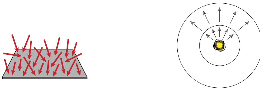
Figure 2.2: Radiant flux \Phi shown in the left image (from Novák [69]). The right image (from Pharr et al. [74]) illustrates radiant flux emanating from a point light source measured at spheres surrounding the light.
