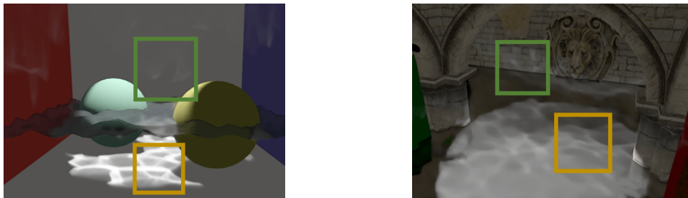
Figure 5.7: Rendering of two scenes with a specular interface producing refractive (emphasized by orange rectangle) and reflective (emphasized by green rectangle) caustics. The reflective shadow maps resolution is 2048 \times 2048 with up-to 2 million photons. ( Renderings by Meenrattanakorn et al. [54]. )
