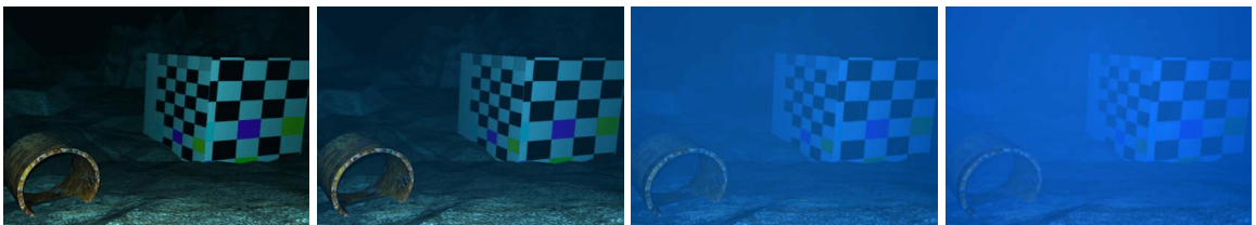
Figure 4.7: Renderings with increasing turbidity from left to right, caused by the increased concentration of scattering particles. ( Renderings from Sedlazeck et al. [46] ).
