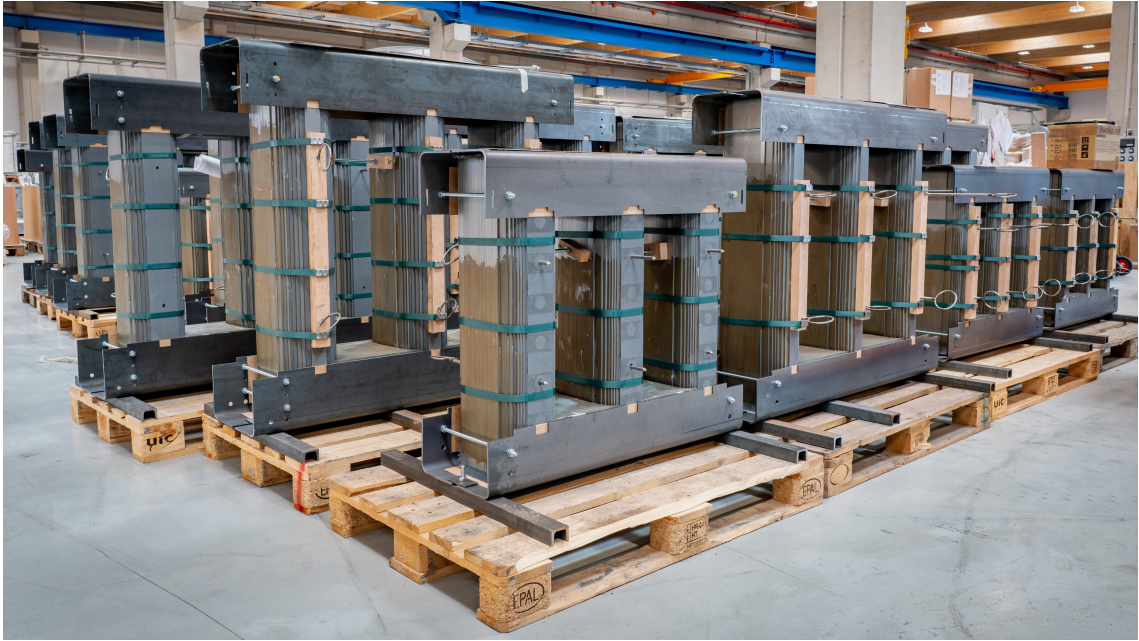
Fig. 6.3: Storage area with assembled transformer cores awaiting winding installation at Elpro-Energo Transformers s.r.o. [18].
