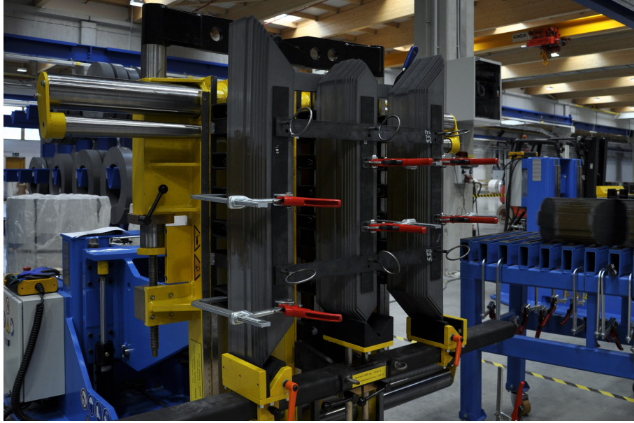
Fig. 3.7: Core building performed on a special rotating hydraulic table for vertical assembly, adapted from [18].
