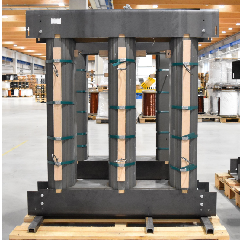
Fig. 2.3: Assembled transformer core with clamping beams prepared for winding installation, adapted from [18].
