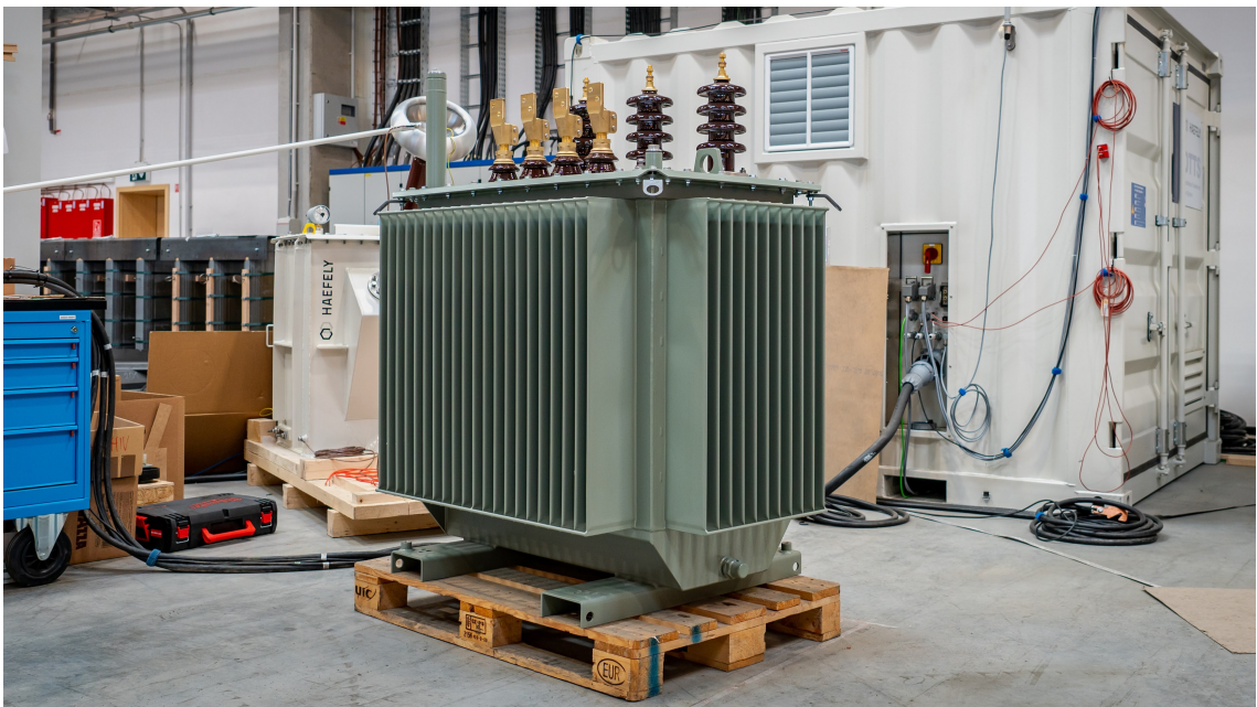
Fig. 6.4: Completed transformer positioned in the testing laboratory at Elpro-Energo Transformers s.r.o. [18], where the no-load test is conducted.
