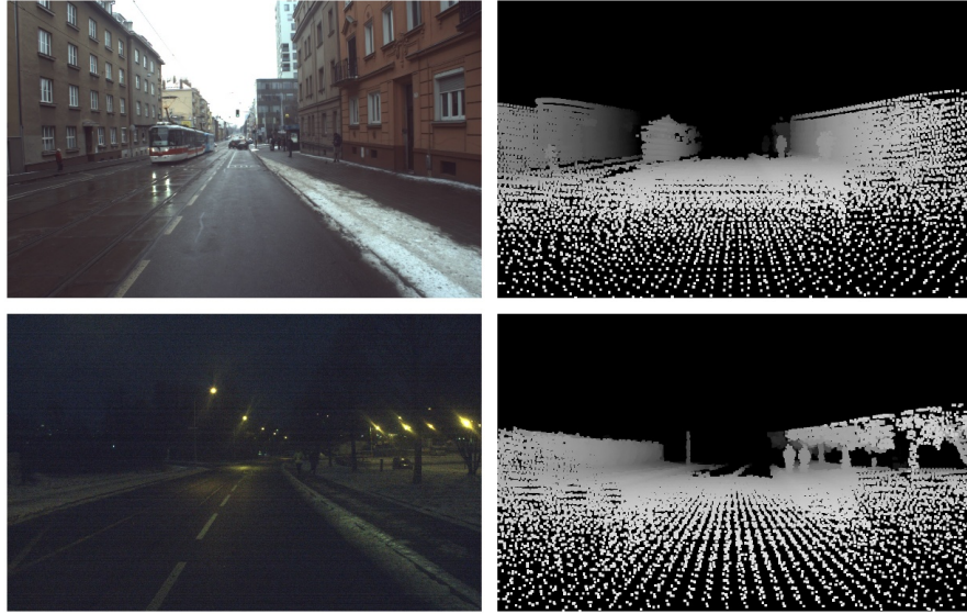
Fig. 2. The example of the RGB images (left) with the corresponding depth map image (right) generated by projecting point cloud to camera frame, using the pinhole camera model.
