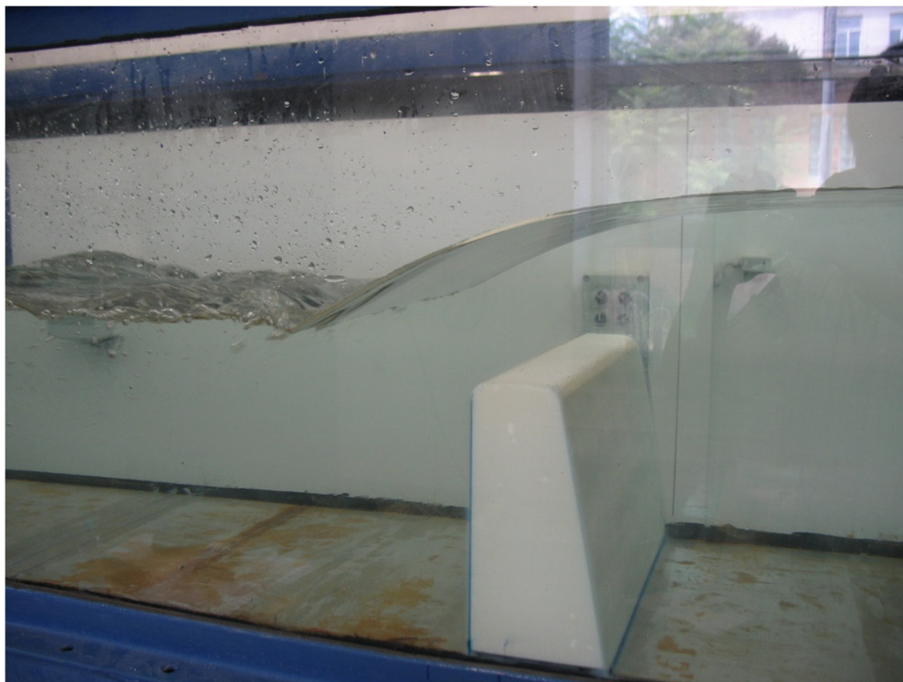
Obrázek 57 - Q = 35 l/s, h = 115 mm, h_z = 62 mm
