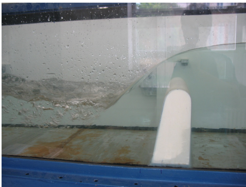
Obrázek 65 - Q = 30 l/s, h = 95 mm, h_z = 7 mm
