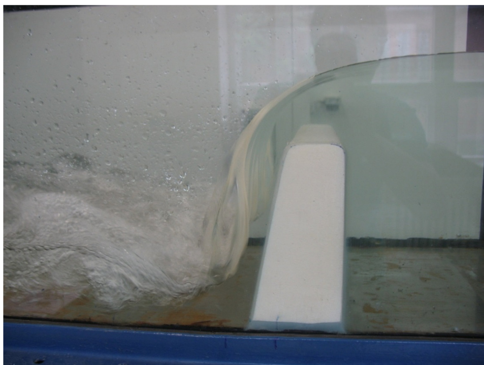
Obrázek 59 - Q = 20 l/s, h = 77 mm, h_z = 0 mm
