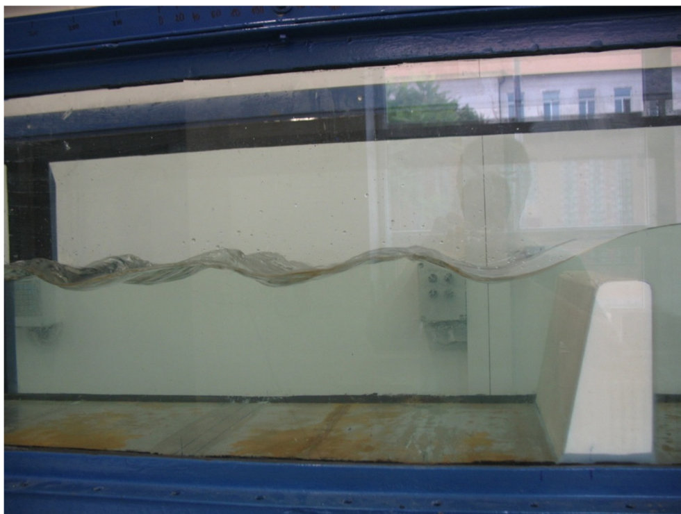
Obrázek 58 - Q = 10 l/s, h = 55 mm, h_z = 26 mm
