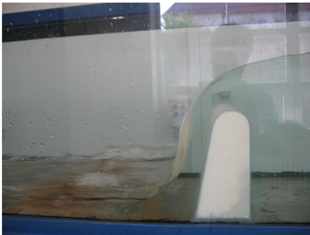
Obrázek 64 - Q = 25 l/s, h = 82 mm, h_z = 0 mm
