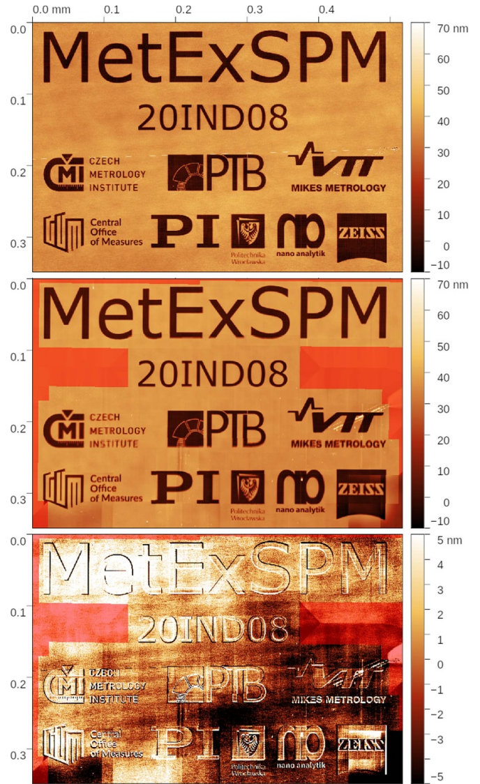
Figure 5. Commercial SPM data stitching compared to NMM results. From top to bottom: NMM reference measurement, stitched data from Dimension Icon and difference between them. Red mask shows the areas that were not measured on Dimension Icon.
