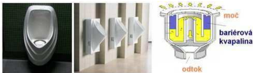
Obr.3.5 Suchý pisoár a) Flickr, b) Kohler Steward c) princip (EcoTrap) [7]
