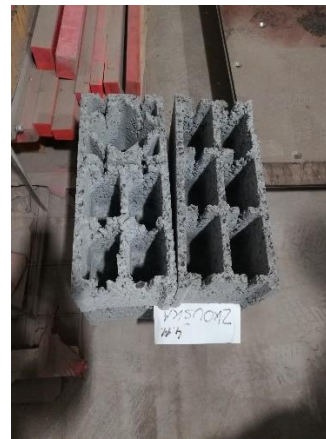
Figure 5. The resulting ultra-lightweight masonry block - after drying.
