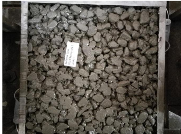
Figure 2. Detail of lightweight concrete surface.
