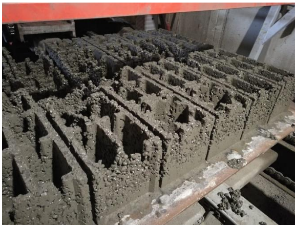
Figure 4. Ultra-lightweight masonry blocks - fresh state after pressing.
