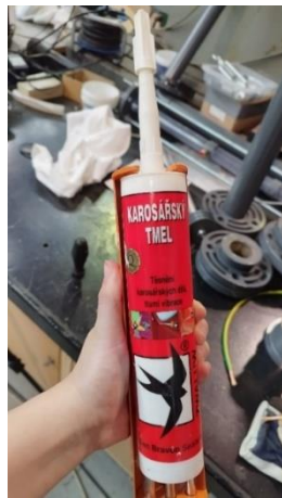
Figure 5-4 Body sealant used to prevent air intake in underpressures
