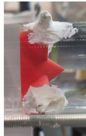
Figure 5-5 Cavitator in water with body sealant applied on the outside of screw connection
