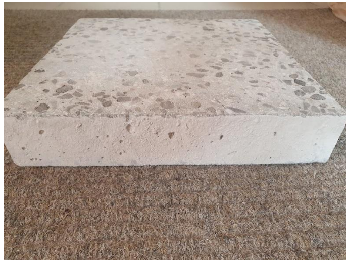
Figure 2. Test specimen for determination of thermal conductivity.
