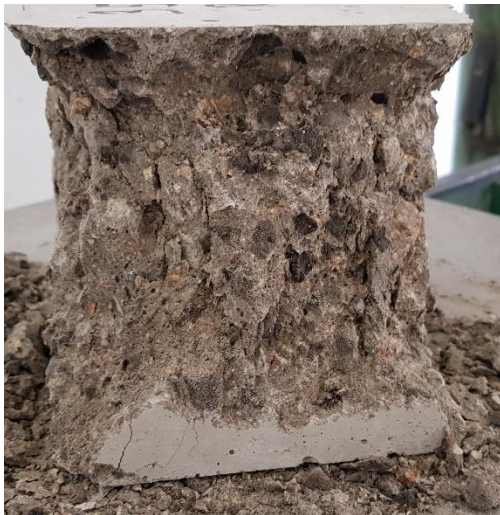
Figure 1. Test specimen after compressive strength test.
