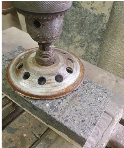
Figure 5. Modification of plate samples for perfect placement in the measuring device.
