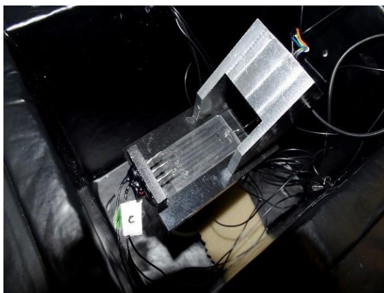
Figure 18 The prepared microfluidic chips connected to the laboratory-made electrophoretic system
