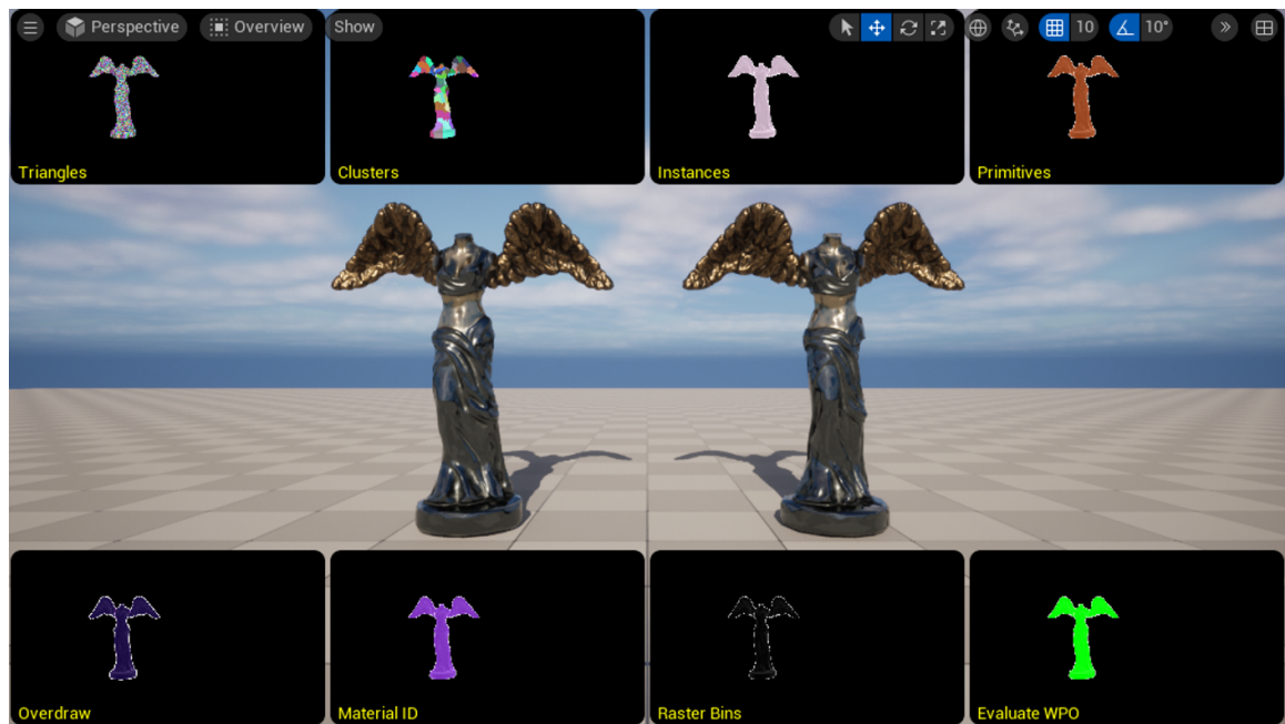
Figure 5.12: Example of Nanite activated on an Actor with different views. Left is a mesh generated from Nanite. Right is the original Static Mesh. Image was taken from [21, Nanite Virtualized Geometry].
