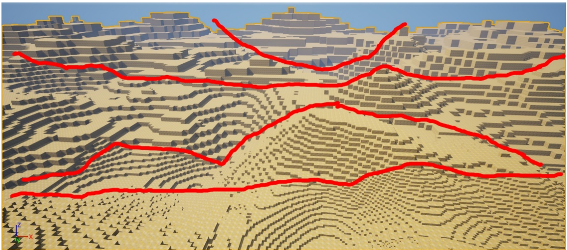
Figure 6.4: Voxel-based environment generated by Voxel Plugin in a showcase level with highlighted LOD transitions.
