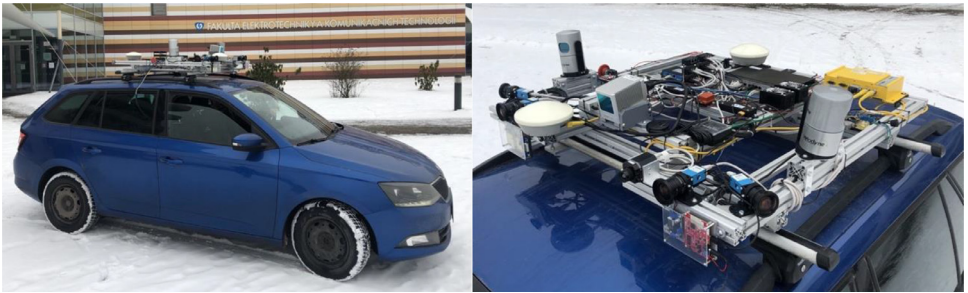
Fig. 1. (left) The Atlas sensory framework installed on the roof of the testing car. Data were recorded in the early February of 2021; (right) Detail sensory framework overview. Four RGB cameras (blue), two side Velodyne scanners and single Livox sensor (all gray), GNSS RTK receiver (yellow) with pair of differential antennas (white), Xsens IMU (orange) in the center, and the FMCW radar (red) in the front of the framework.
