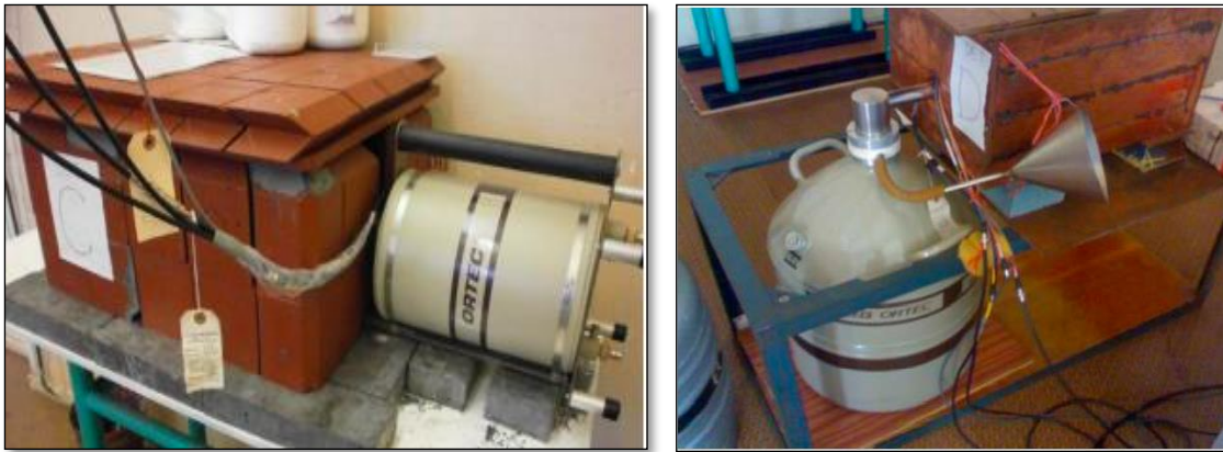
a) b) Fig.5.10. a) HPGe is ORTEC detector. b) Dewar filled with liquid nitrogen.
