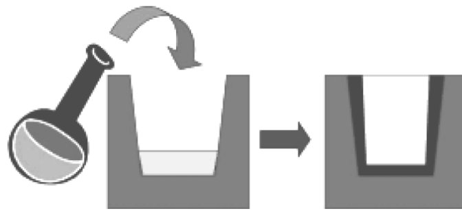
Fig. 2.20. Scheme of the sequential slip casting [15].
