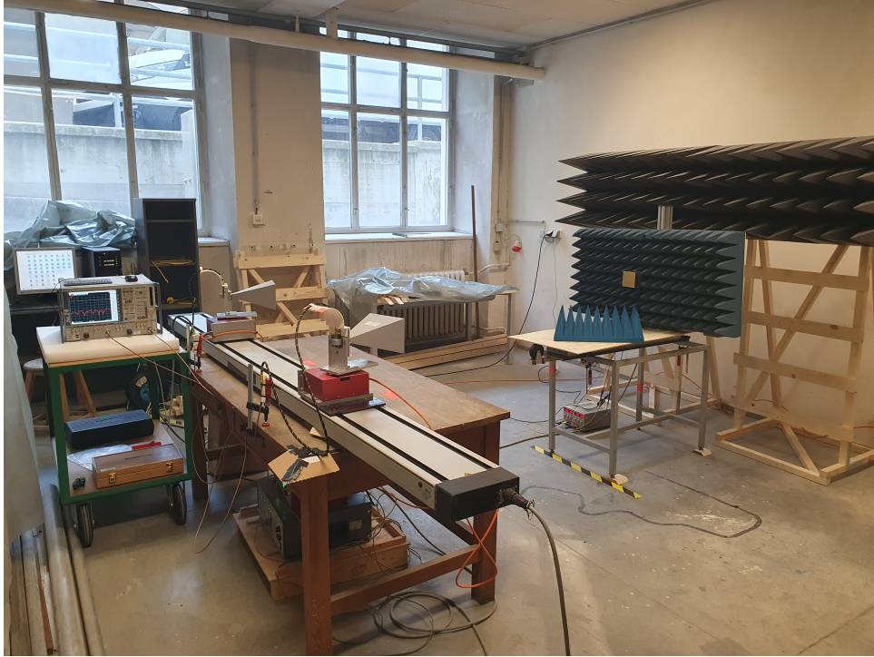
Fig. 3.17: Photo of the used testbed for the RIS. The RIS is attached to a stand that can move on a linear spindle drive. The stand has a backboard with absorbers (dark blue). The DACs controlling the RIS modules are placed behind this backboard. The supply voltage for the DACs is taken from a power supply placed on the floor. More absorbers are used on the spindle drive (light blue in front of the RIS) and on special rack behind the RIS stand (dark gray). The vector network analyzer ZVA 24 from Rohde & Schwarz is connected to two horn antennas that can be rotated and moved via spindle and rotation drives. Lastly, the whole testbed is connected to a PC for automated measurements.
