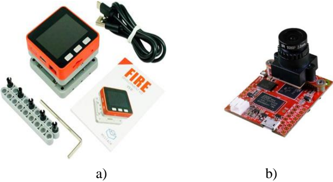
Figure 2: a) M5Stack module b) OpenMVH7 Plus camera
