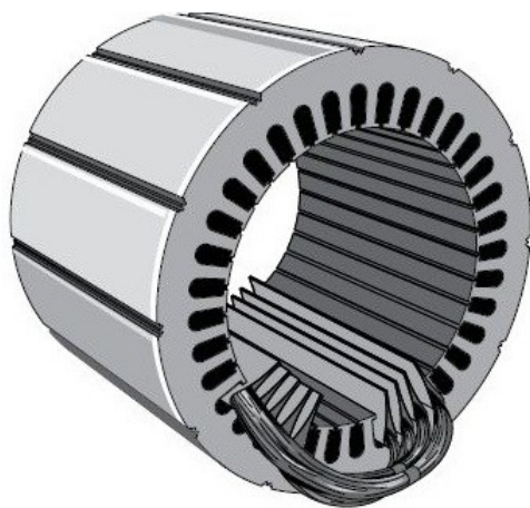
Stator Windings Partially Completed
