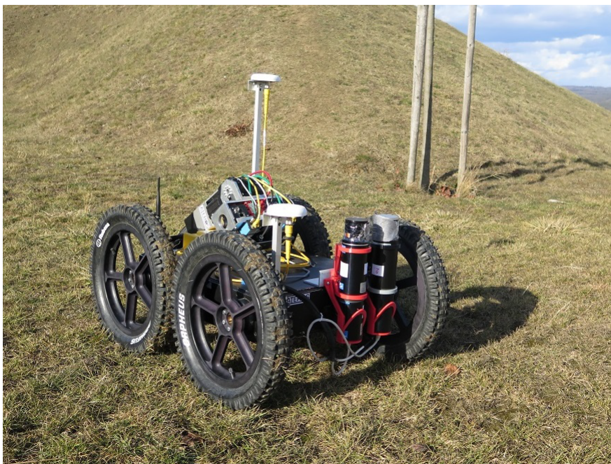
Fig. 2.5: Robot Orpheus-X3 carrying equipment for gamma radiation measurement
