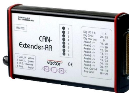
Obr. 38 CAN - Extender – AA [2]
