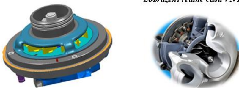
Obr. 17 VNT regulace turbodmychadla [7]
