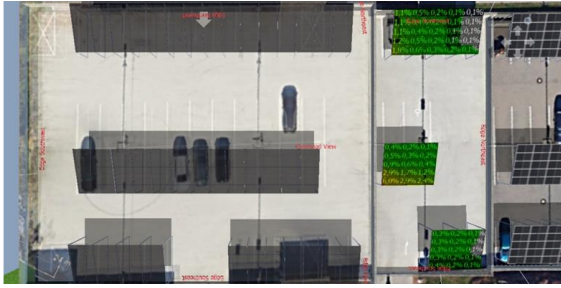
Fig. 13. View of shading analysis of designed solar carport in CESA parking house - second area, maximum shading 6% (one panel), 2.9%
