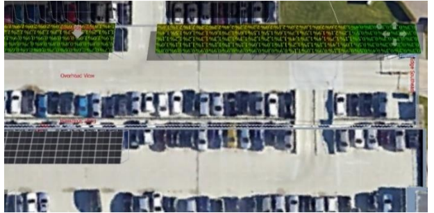
Fig. 10. View of shading analysis of designed solar carport in T12- middle area car park other side, maximum shading 2.4%
