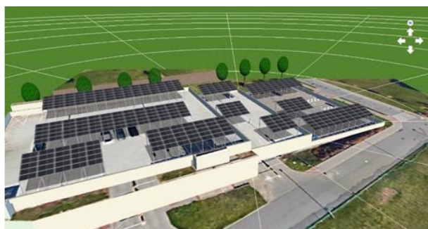
Fig. 6. Sketch of the designed solar carport in car parks CESA
