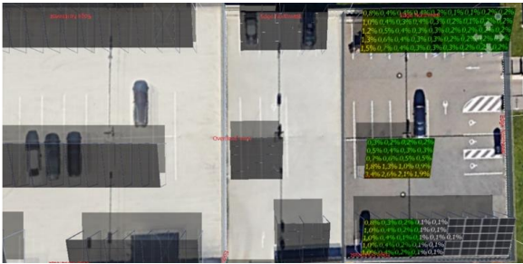
Fig. 14. View of shading analysis of designed solar carport in CESA parking house - third area, maximum shading 3.4%
