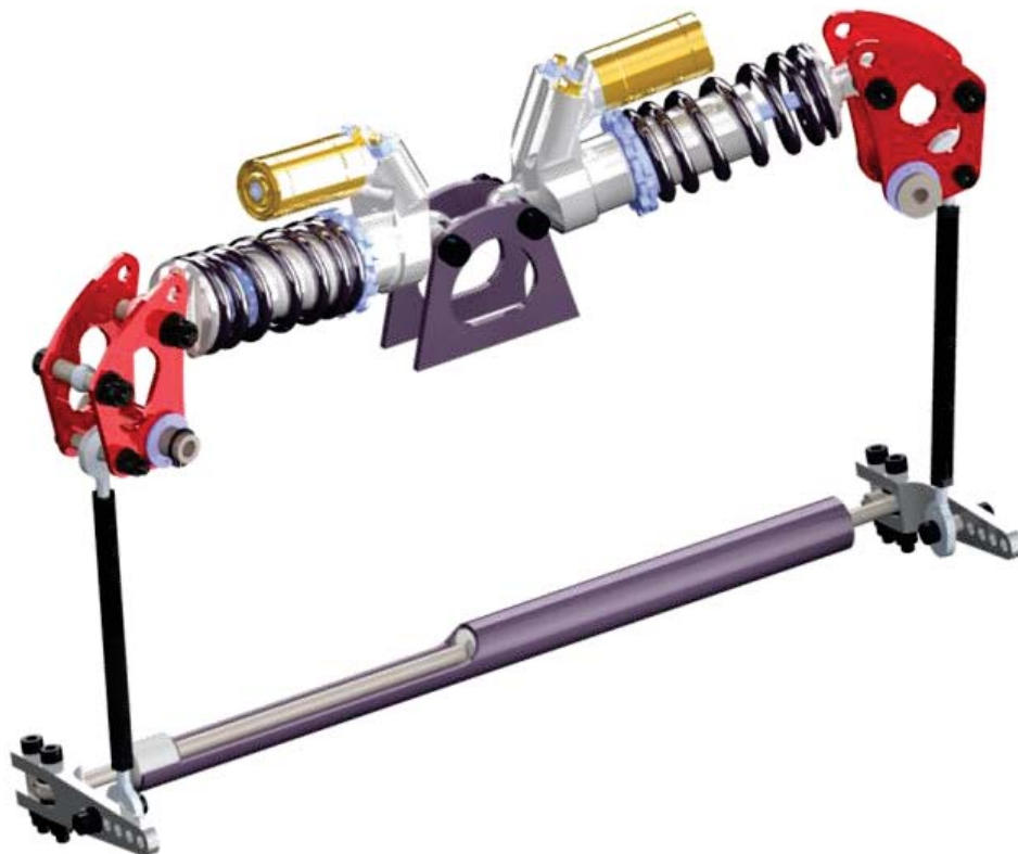
Figure 5 21 Dragon 3 Rear suspension assembly. Anti-roll bar was fitted into one of chassis tubes
