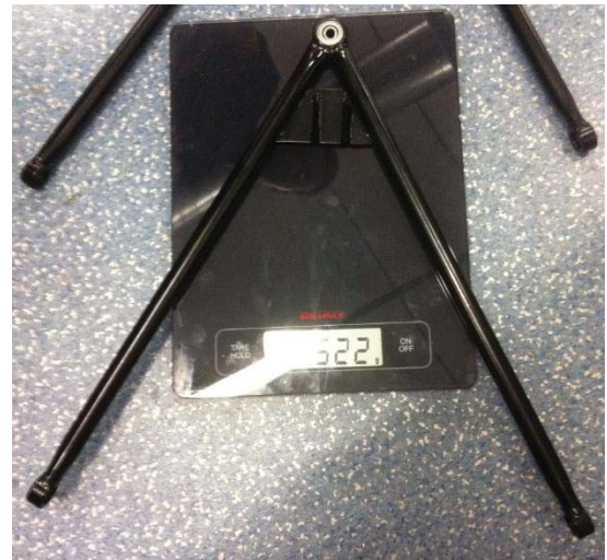
Figure 5 16 Difference of weight is 210 grams. This was considered as a big improvement as this is more than 40 % of weight reduction
