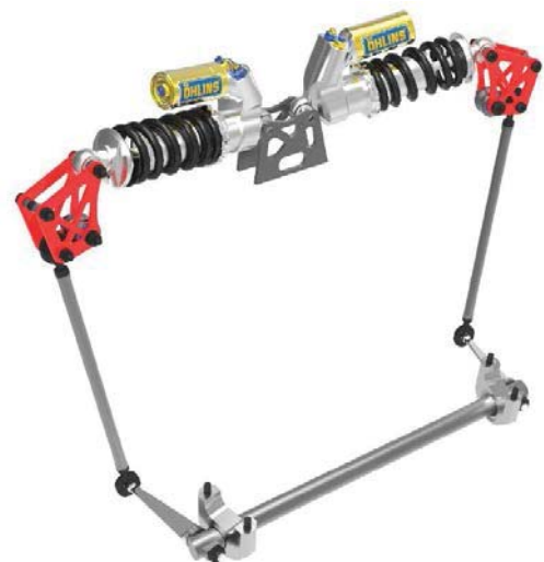
Figure 5 23 Dragon 4 rear suspension assembly with new generation anti-roll bar solution
