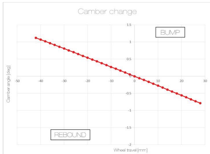
Figure 4 60 Camber change or rear suspension
