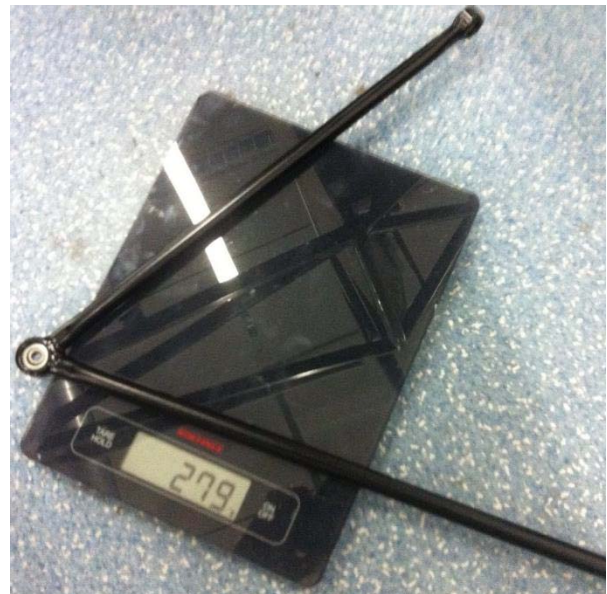
Figure 5 19 Dragon 4 rear upper wishbone is 45 % lighter.
