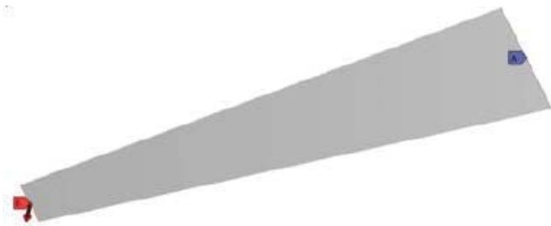
Figure 5 28 Boundary conditions for soft blade position. Force is acting perpendicularly to blade plane
