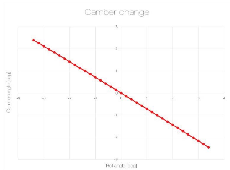
Figure 4 66 Camber change in roll. This try to satisfy tyre characteristics.
