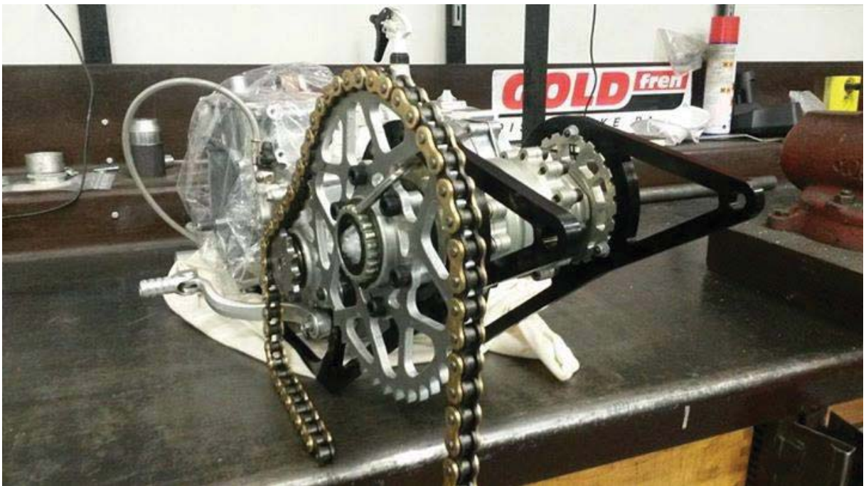
Figure 4 34 the powertrain unit of Dragon 5 is mounted into aluminium holders. This prevents to transform the biggest forces of chain into the chassis.
