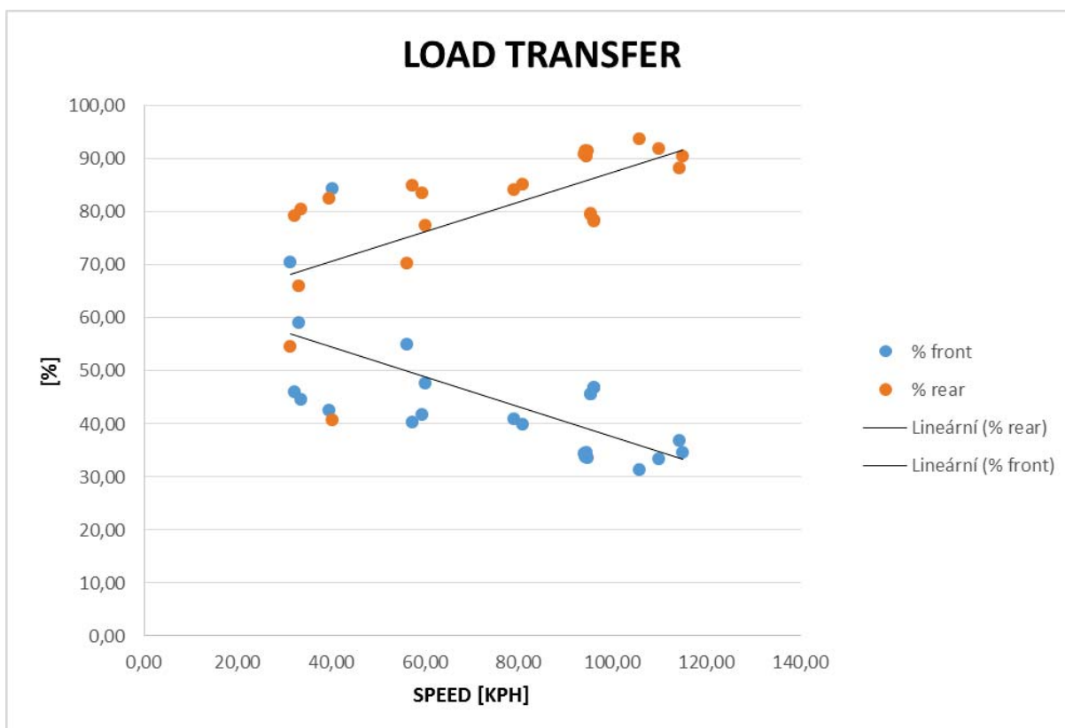
Figure 6.27 aerodynamic load transfer of Dragon 4. At higher speed corners the car would suffer from understeer a lot as the majority of downforce acts at the rear axle. With stiffer springs on the rear axle the car behaviour has been improved significantly.
