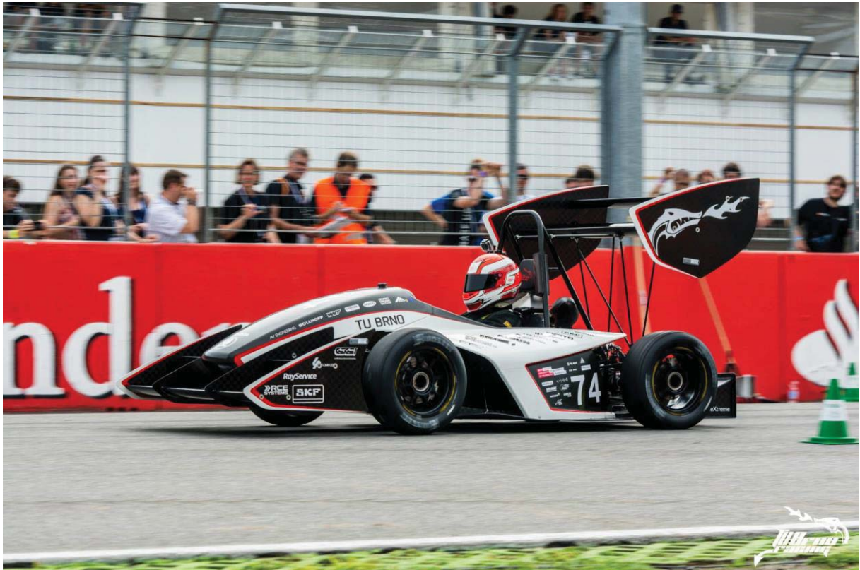
Figure 1. 11 Acceleration event. Different car setup is clearly visible. Wing's flaps are in the "low drag" setup. Ride height is set up according to load transfer. Tyres have different pressure to affect the contact patch and resistance of the car.
