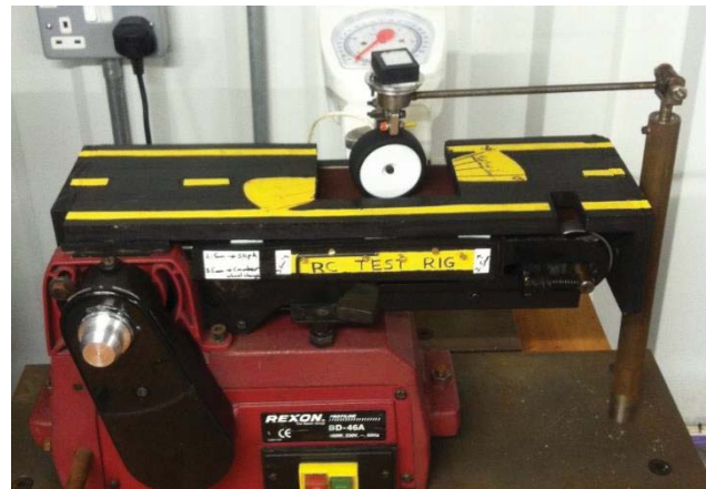
Figure 3. 2 Tyre Test Rig of University of Hertfordshire. Scale 1:10 th for measuring RC car tyres
