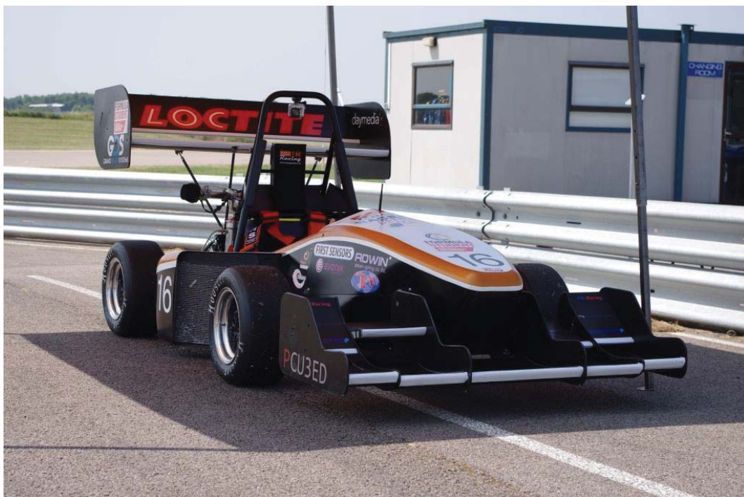
Figure 2. 8 UH 16 was the first winged car. Last UH Racing car with the four cylinder engine
