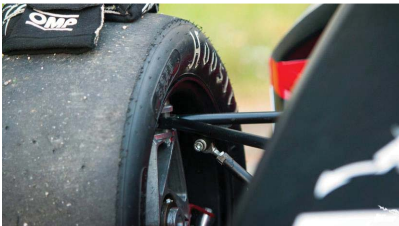
Figure 5 11 Dragon 3 wishbone detail. Material properties were inappropriate and the bearing dimensions were unnecessary over dimensioned
