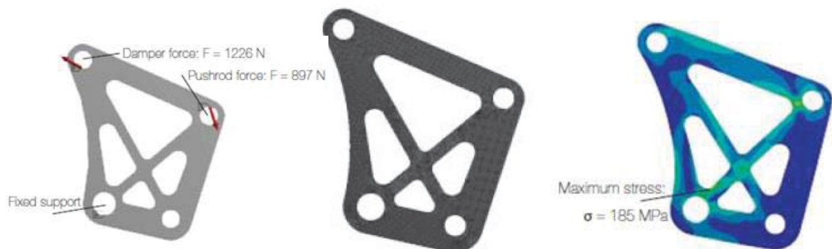
Figure 5 9 Rear Rocker Dragon 4 FEA Analysis.
