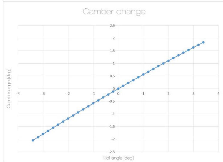
Figure 4 14 Chamber change of suspension is important from the tyres point of view. It is important to keep the tyre in the ideal position as much as possible. Here the camber trust is taken into account as well.
