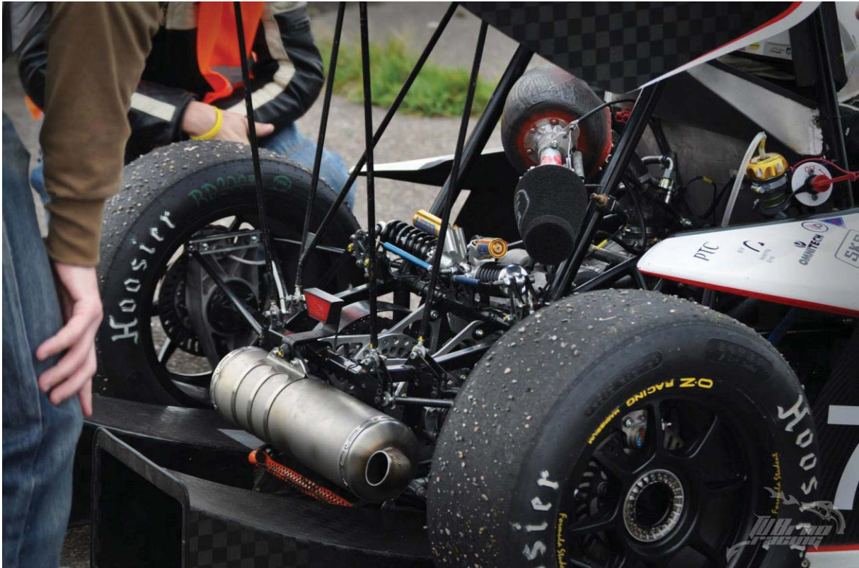
Figure 4.33 Dragon 4 rear suspension layout. The mass of space frame around differential unit was eliminated for Dragon 5
