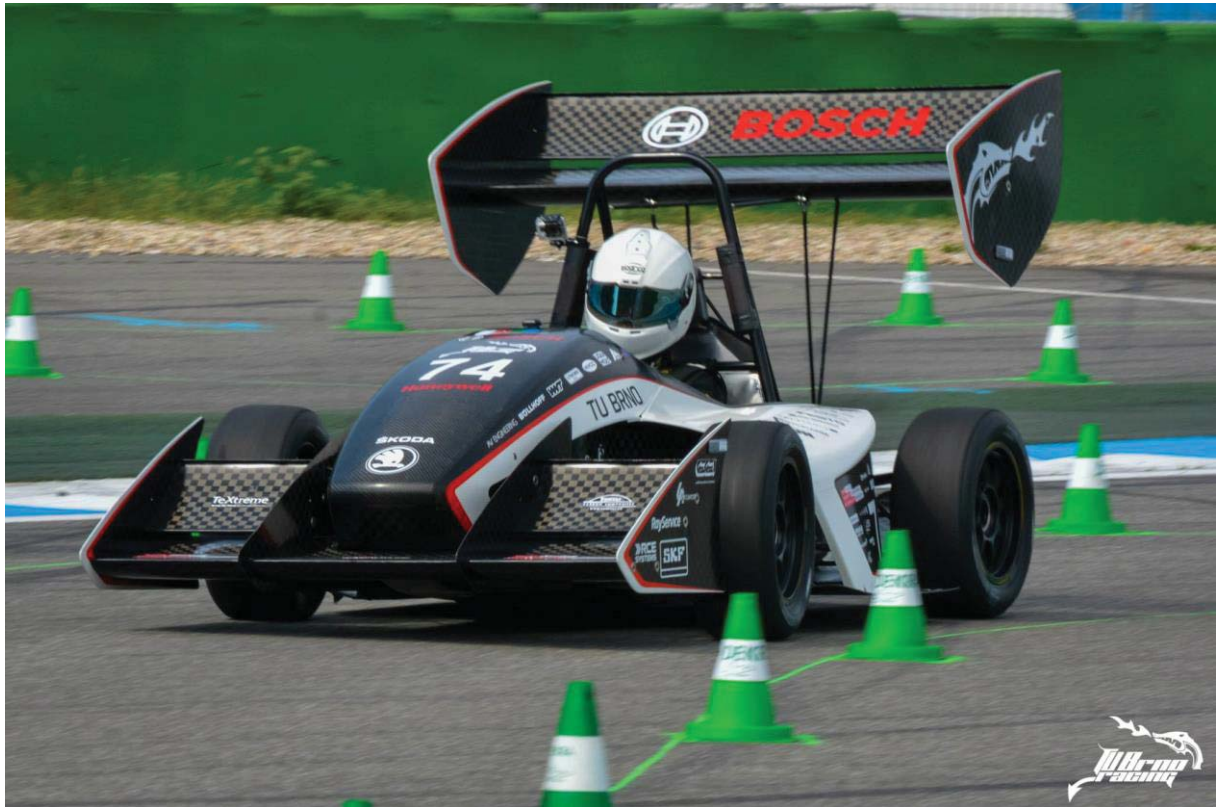
Figure 1. 13 Autocross Event at the Formula Student Germany. Setup is changed from the acceleration to autocross. As the driver has only 2 laps to establish the time, car has to be set up according to this conditions. Biggest challenge is to heat the tyres.
