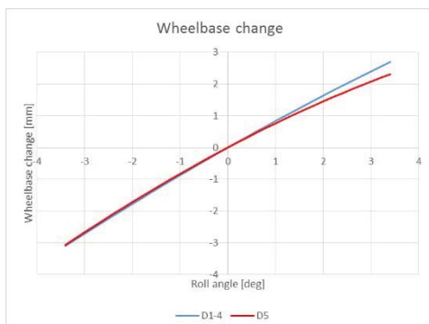
Figure 4 86 wheelbase change is almost identical.
