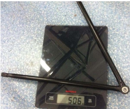
Figure 5 20 Dragon 4 rear upper wishbone in configuration with bigger tubes cross section dimensions.
