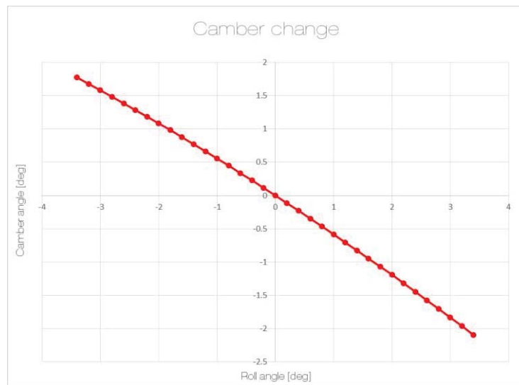
Figure 4 50 In roll it is important to allow tyre to have as big as possible contact patch all the time.
