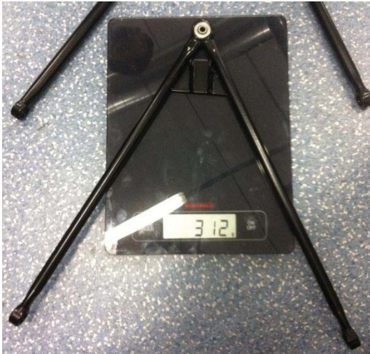
Figure 5 17 Dragon 4 lightweight version of front upper wishbones. The pull rod attachment point is visible.
