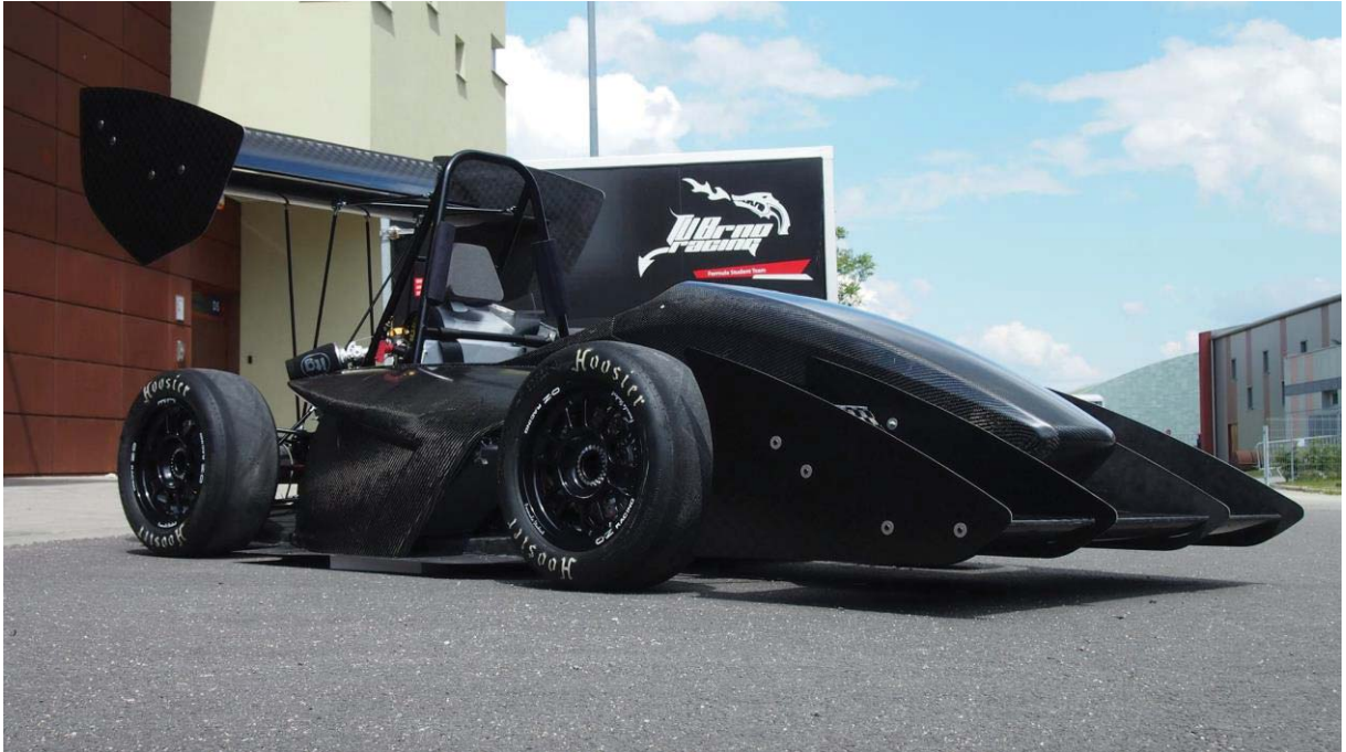
Figure 2. 5 Dragon 4 before season 2014. First test day 31st of May. The missing livery shows how much composites were used to save the weight. Dragon 4 is the first winged car. Even with the wings it is 15% lighter than Dragon 3 without wings.
