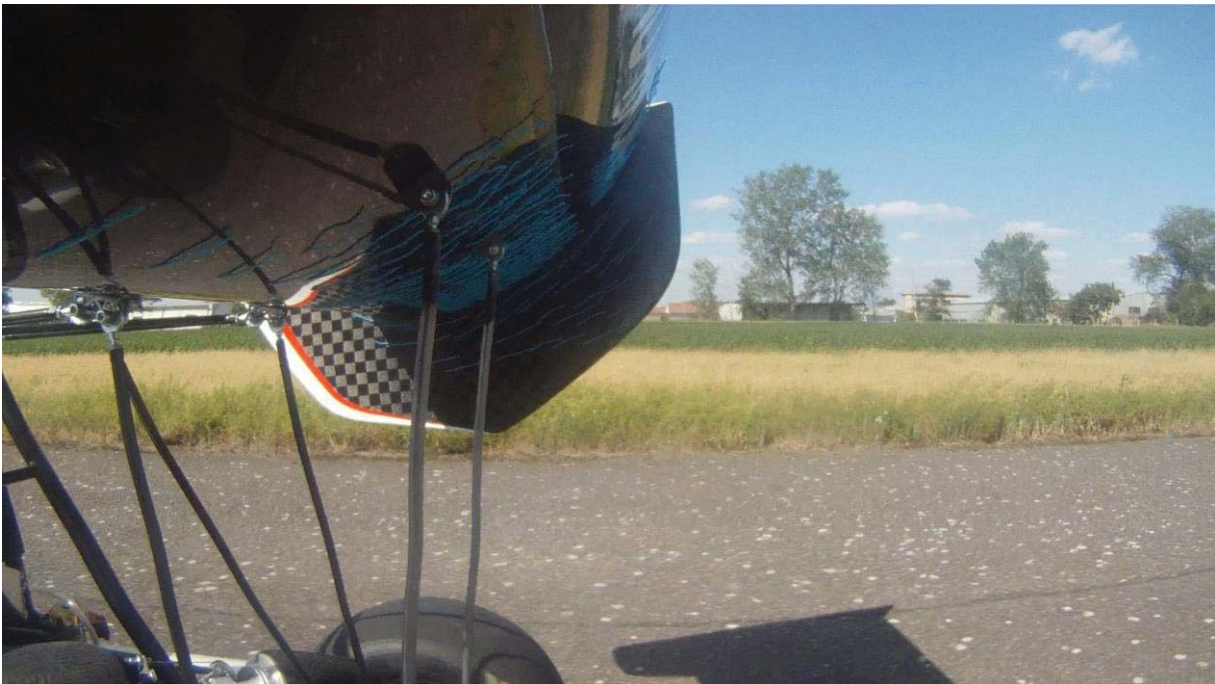
Figure 6 29 Go Pro camera mounted on rear wing end plate provides really important set of data as well. Boundary layer of this wing is really good. Cotton strings were stable and straight during every speed level.
