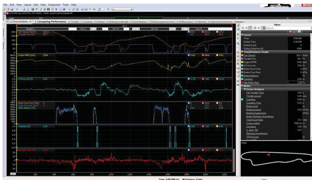
Figure 6.1 MoTeC i2 pro software with example data. Speed trace, throttle position pedal trace, engine RPM, lateral acceleration, brake pressures or coasting calculation is shown driver to improve his or her time.
