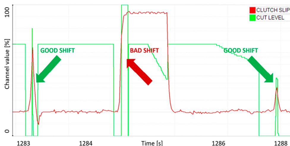
Figure 5. Identification of shifting delay locations using CUTLEVEL and CLUTCHSLIP channels.
