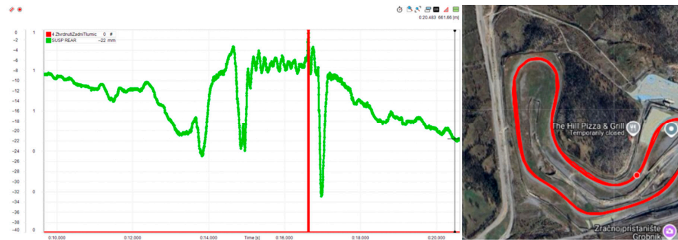
Figure 11. Rear suspension bottoming detection with a marked exact point on the track, where it occurred (right).
