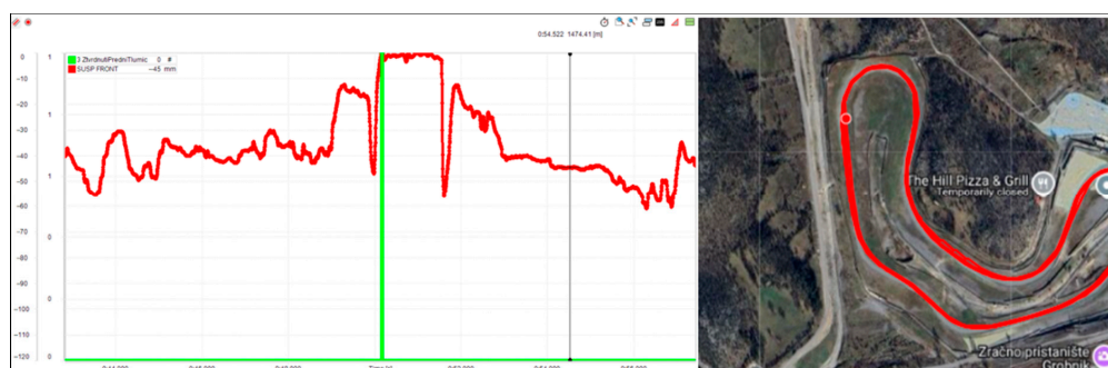
Figure 10. Front suspension bottoming detection (left) with marked exact point on the track, where it occurred (right).
