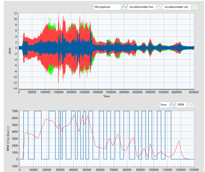
Fig. 2. Top: analog data from microphone and accelerometers, bottom: speed profile (red line) and error presence (blue line) of the PMSM.
