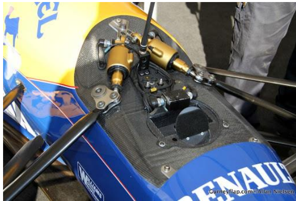
Pic. 2.3 Detail of Williams FW15C Formula 1 car hydraulic suspension [19]
