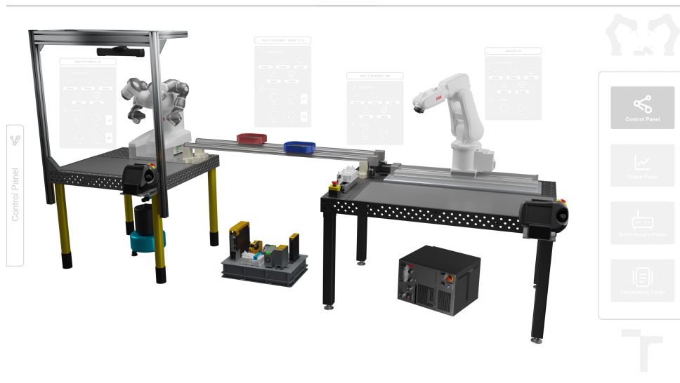
Figure 5.5: An overview of the home screen structure of the web-based Human-Machine Interface (HMI) created using B&R Automation technology, known as mapp View.
