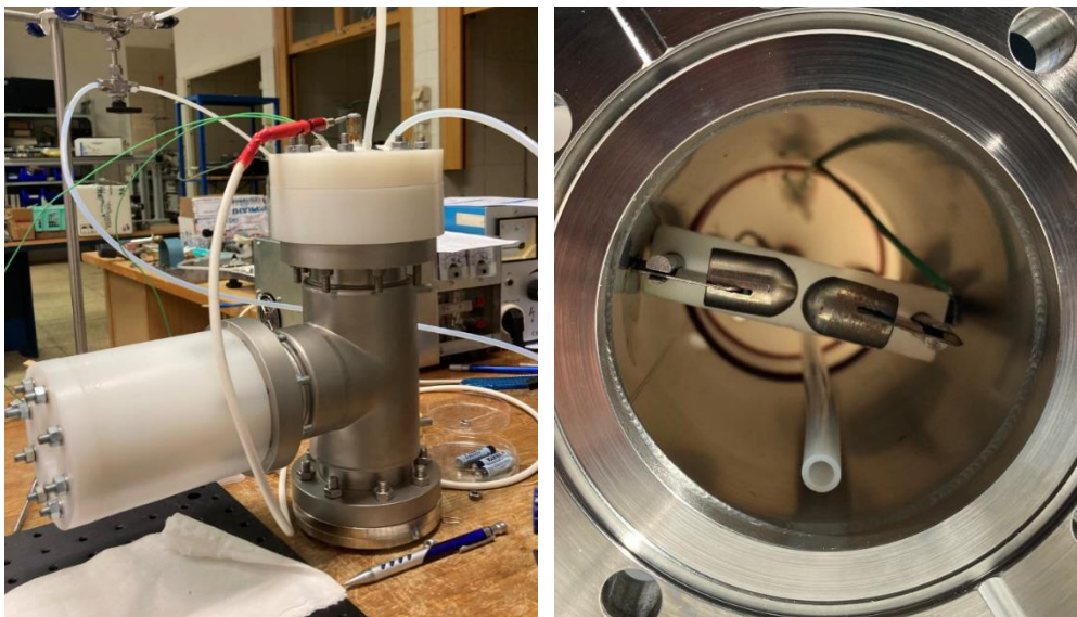
Fig. 17 Stainless steel high vacuum reactor used in experiments.
