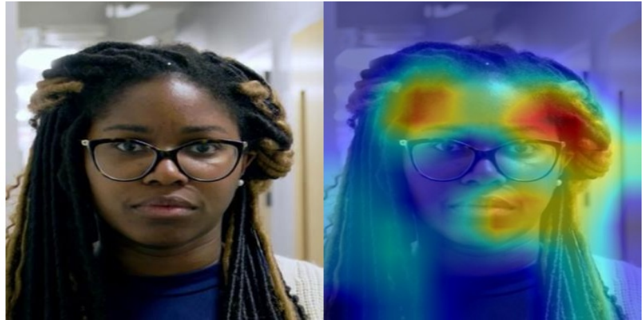
Figure C.2: Heatmap example with 0% deepfake prediction score. Genuine correctly classified as genuine by detector.
