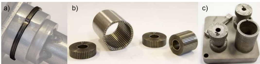
Fig. 31 Shape approach of magnetic circuit time response decrease
