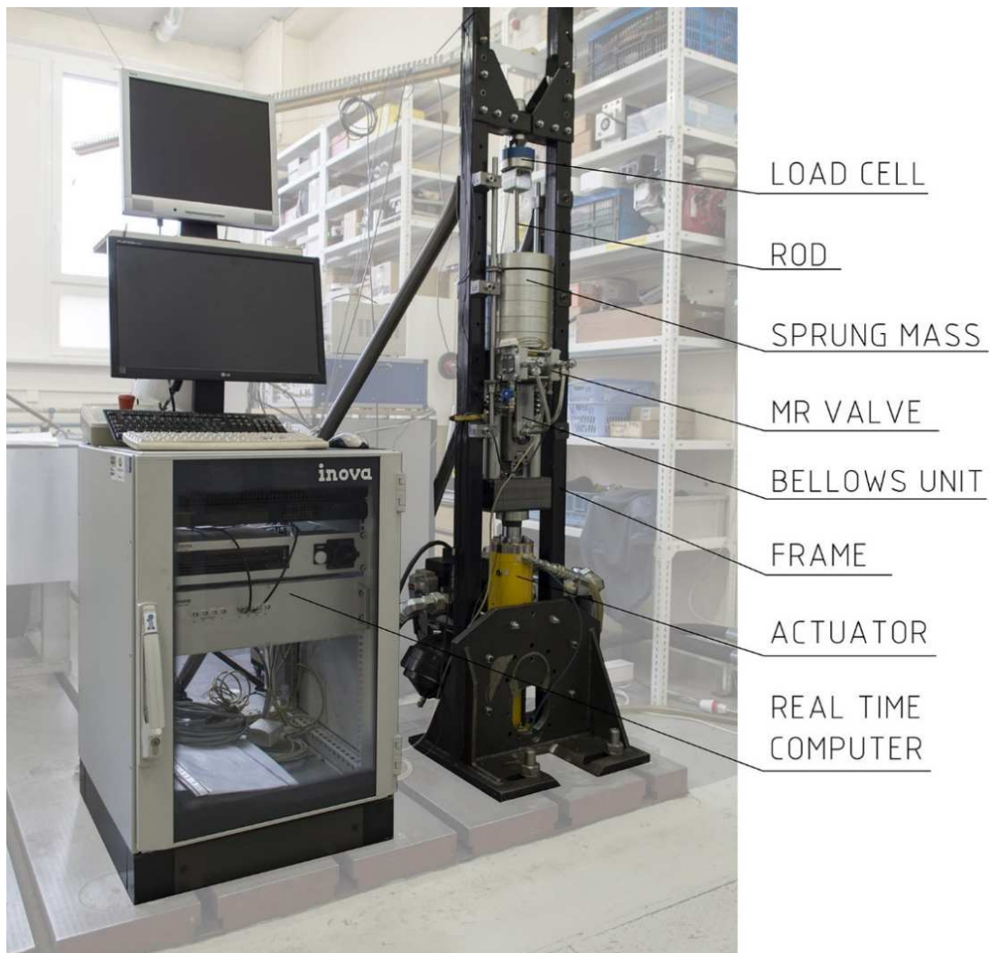
Fig. 25 Demonstrator configuration for the F-v dependency measurement
