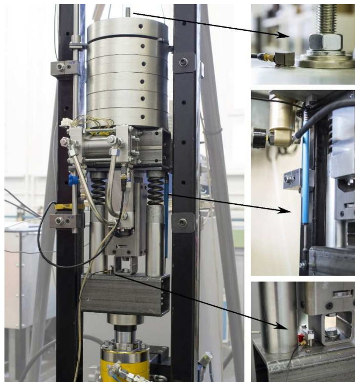
Fig. 24 Demonstrator for the experimental strut vibration isolation properties verification
