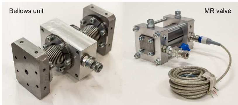
Fig. 23 Important parts of the experimental MR strut
