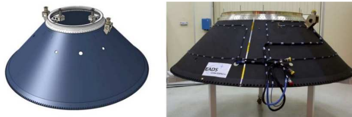
Fig. 3 ESA adapters: PAS 937C (left) [8] a PAS 1194C (right) [9]
