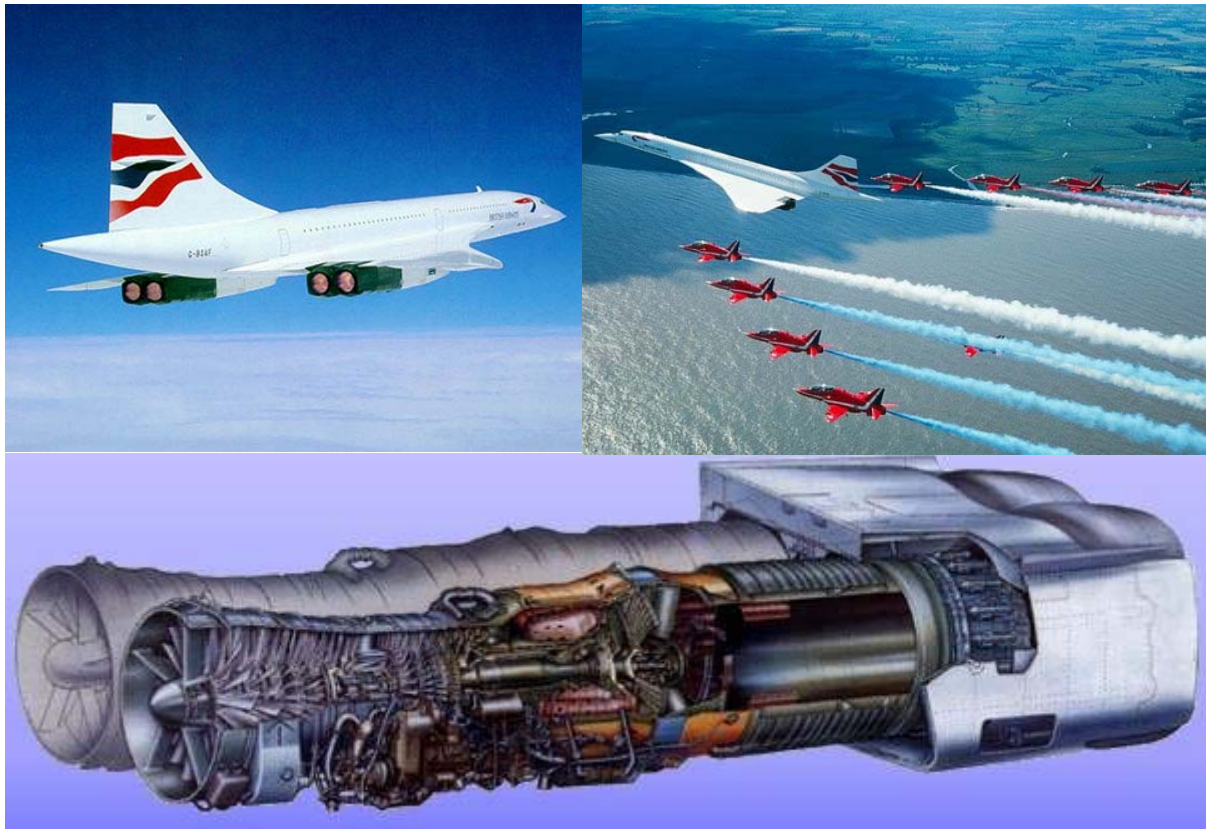
Obr. 4.5 Concorde se 4 motory Rolls Royce/SNECMA Olympus 593 MK610 turbojet [25] [26] [27]
