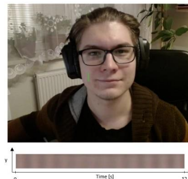
Figure 1: Pulsing skin color after exaggeration. Green line shows the section which has been expanded onto the time axis below the picture
