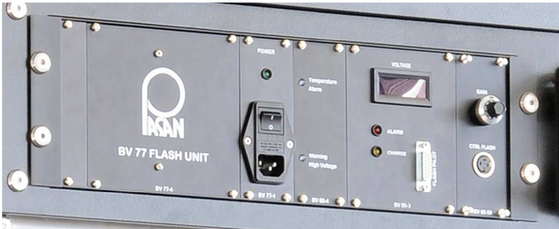
Fig 4: electronic cards on the flash generator
