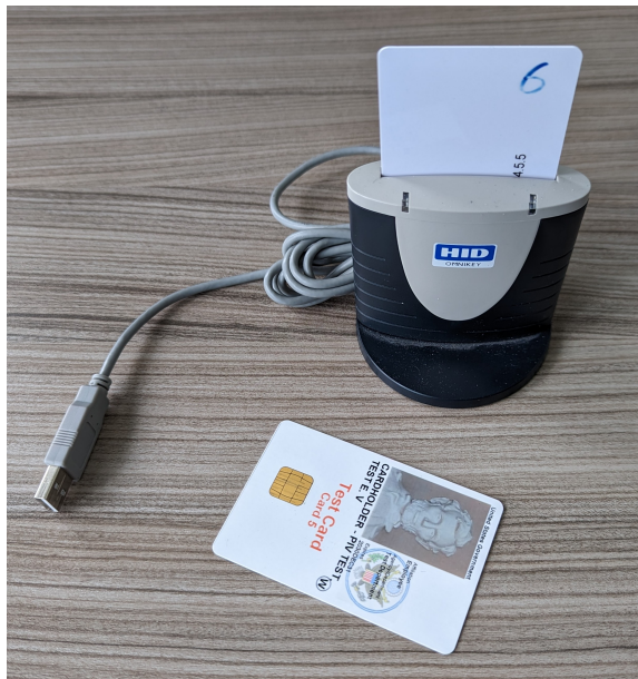
Figure 2.1: USB smart card reader with one smart card inserted and a second one placed in front of it
