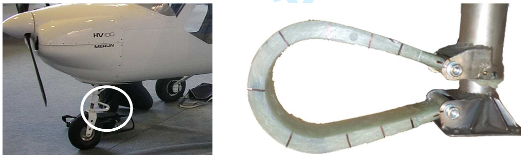
Figure 15 Merlin 103 nose wheel spring.
